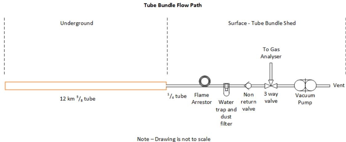
**Figure 1: Tube Flow Path**
