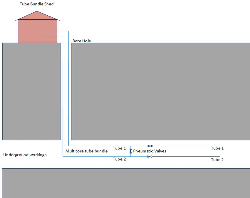
Figure 3: Parallel Flow Path
