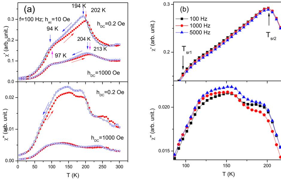
FIG. 2. Temperature dependences of the ac magnetic susceptibility of  $\text{DyFe}_{11.2}\text{Nb}_{0.8}$  as measured under: (a) DC fields  $h_{\text{DC}} = 0.2$  Oe ( $h_{\text{ac}} = 10$  Oe;  $f = 100$  Hz) and  $h_{\text{DC}} = 1000$  Oe and (b) with different ac frequencies of  $f = 100$  Hz,  $f = 1000$  Hz,  $f = 5000$  Hz ( $h_{\text{ac}} = 10$  Oe;  $h_{\text{DC}} = 0.2$  Oe; warming process). The warming (red) and cooling (blue) directions are indicated by arrows in Figure 2(a).
