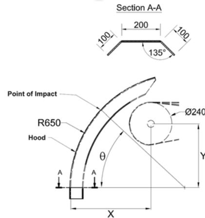
**Figure 2** Detail of conveyor transfer hood
