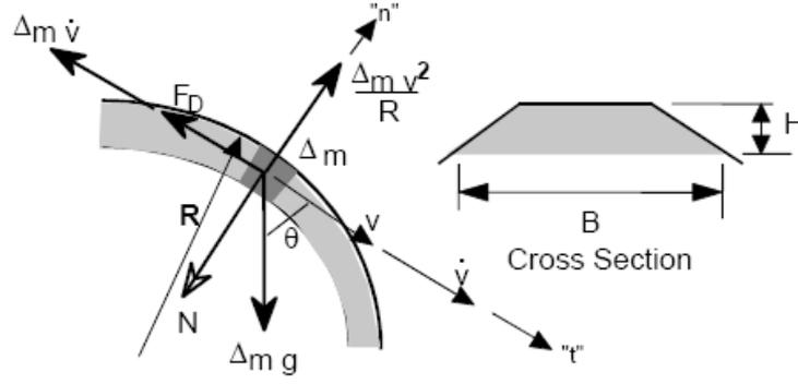
**Figure 4** Force diagram for the inverted curved chute [2]
