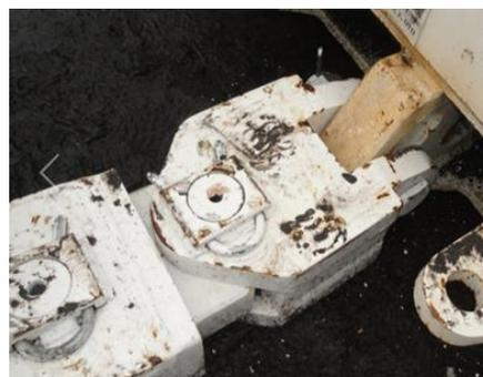
Figure 3: Clevis and attachment to AFC
