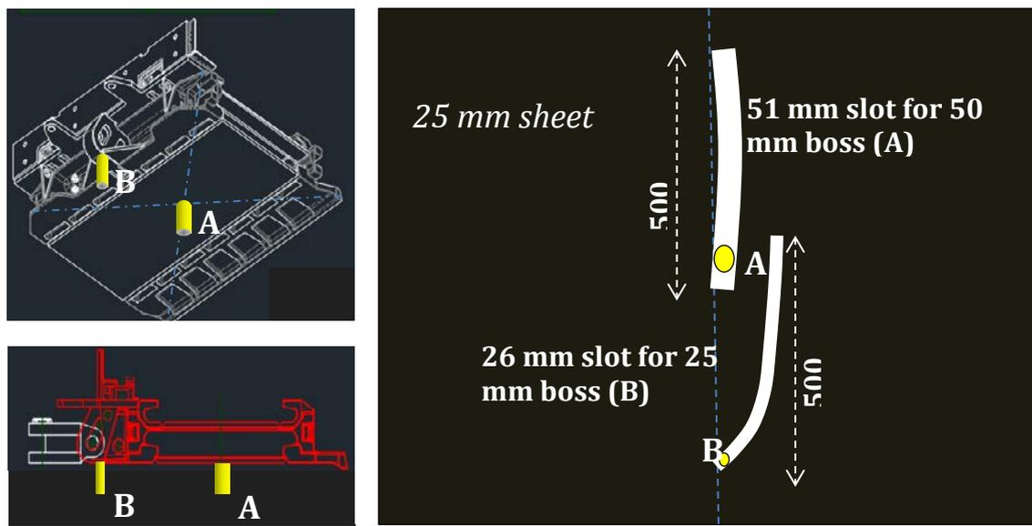
Figure 6: Conceptual design of rig to test pan snake
