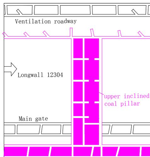
Figure 4: The relative location of LW12304 and upper inclined coal pillars
