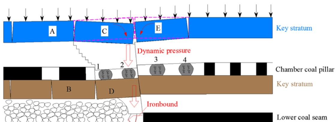
**Figure 7: Overburden rock block structure and load transfer when there were chamber coal pillars ahead of the longwall face**
