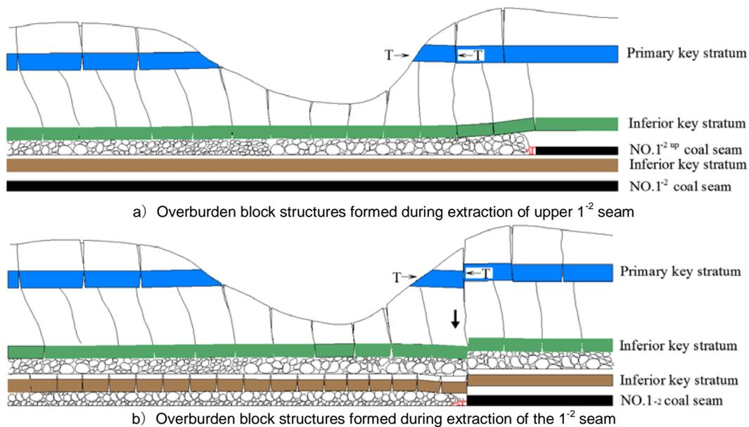
**Figure 3: Movement of rock blocks when the coalface was beneath the valley slope**
