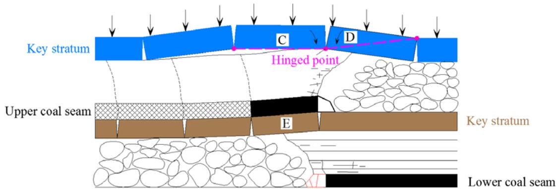
**Figure 5: Strata block structures and movements when upper a coal pillar was undermined**
