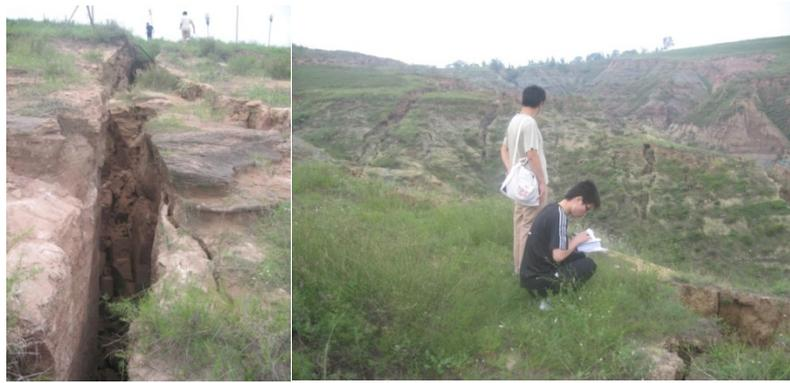
**Figure 2: Surface cracks with scarps on the slope of the valley**
