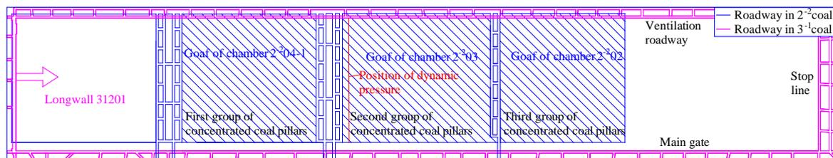
**Figure 6: Layout of the longwall 31201 and upper coal seam chambers**
