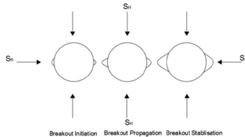
**Figure 4: Borehole breakout formation**
