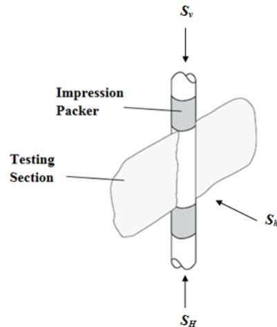
**Figure 1: Conventional hydraulic fracturing (after Lakirouhani, *et al.*, 2016)**
