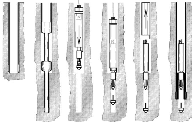
Figure 3: Overcoring procedures (Ljunggren, *et al.*, 2003)
