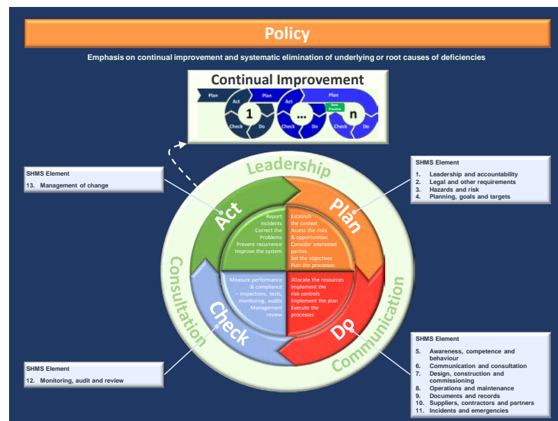
Figure 3: Illustration of how elements of an SHMS fit into the PDCA framework
