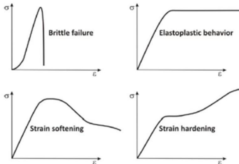
**Figure 1: Different types of stress-strain curves for different rock behaviors under various loading conditions**
