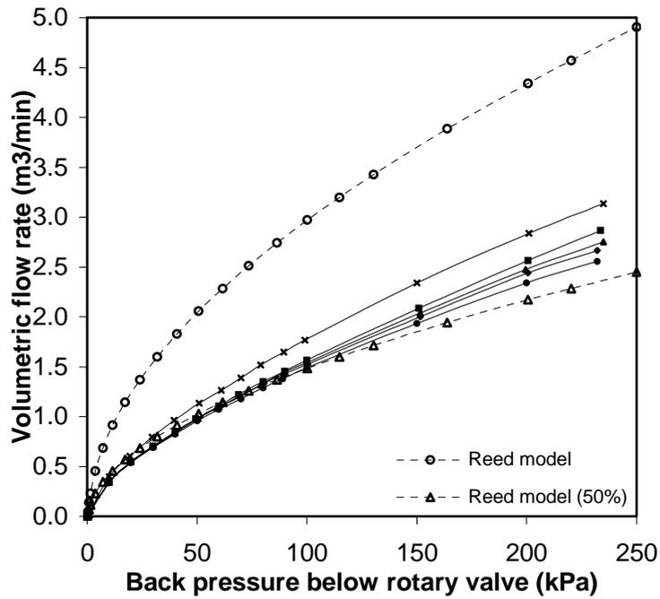
Figure 10 Comparison of Reed model with ZGR 250 experimental results
