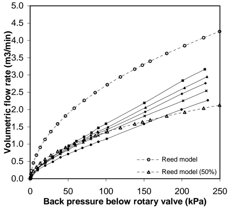
Figure 11 Comparison of Reed model with ZGH 320 experimental results
