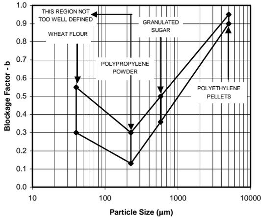
Figure 6 Static blockage factor [4]
