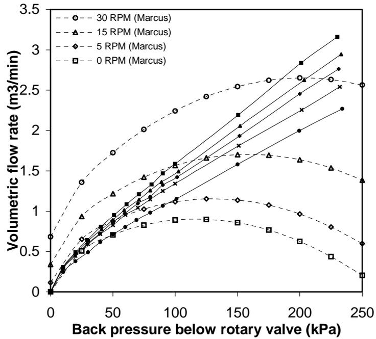
Figure 5 Comparison of Marcus model with ZGH 320 experimental results
