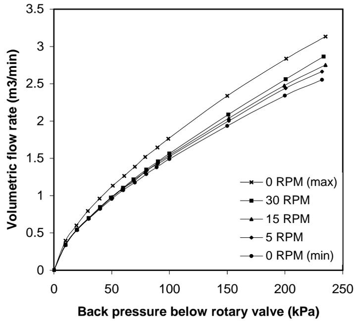
**Figure 2** Experimental air leakage from Waeschle ZGR 250 rotary valve
