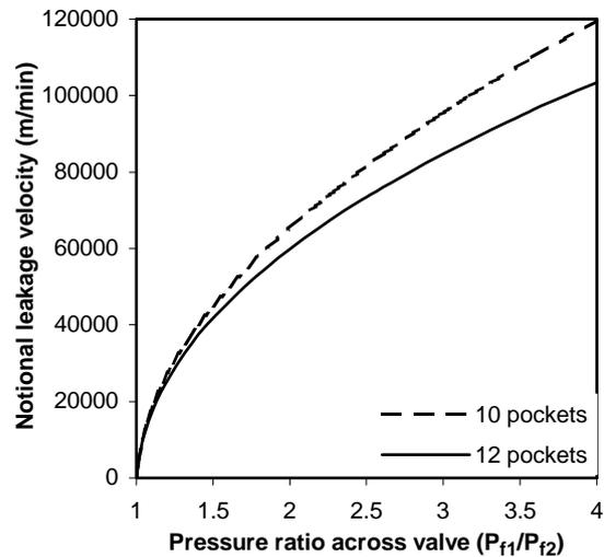
Figure 9 Extrapolated leakage velocity versus pressure ratio for 10 and 12 pocket rotary valves
