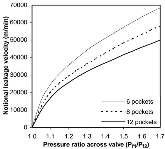
Figure 8 Leakage velocity versus pressure ratio for 6, 8 and 12 pocket rotary valves
