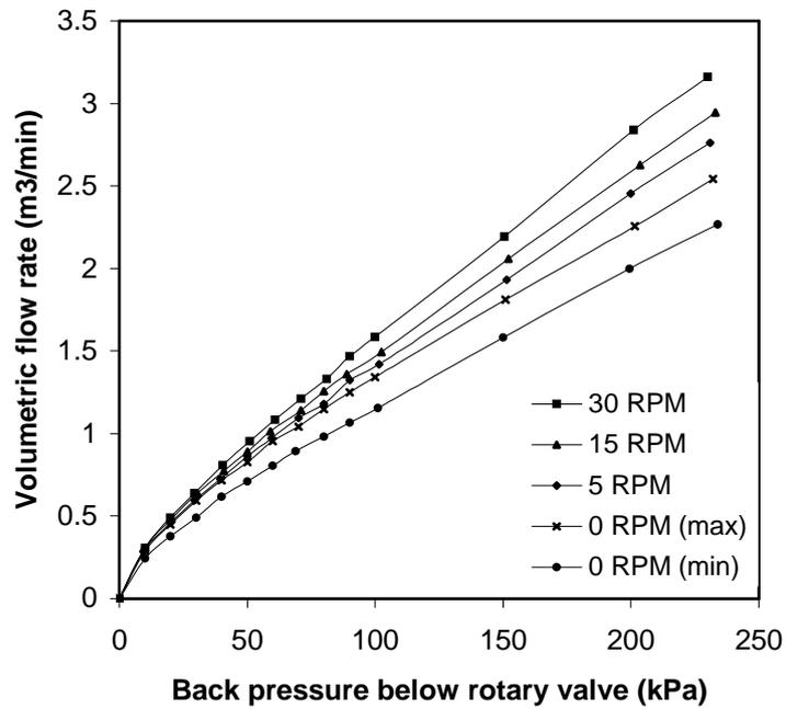
**Figure 3** Experimental air leakage from Waeschle ZGH 320 rotary valve
