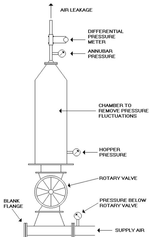
**Figure 1** Diagrammatic representation of Waeschle ZGR 250 rotary valve test rig arrangement
