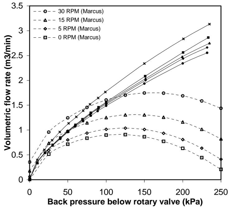
Figure 4 Comparison of Marcus model with ZGR 250 experimental results
