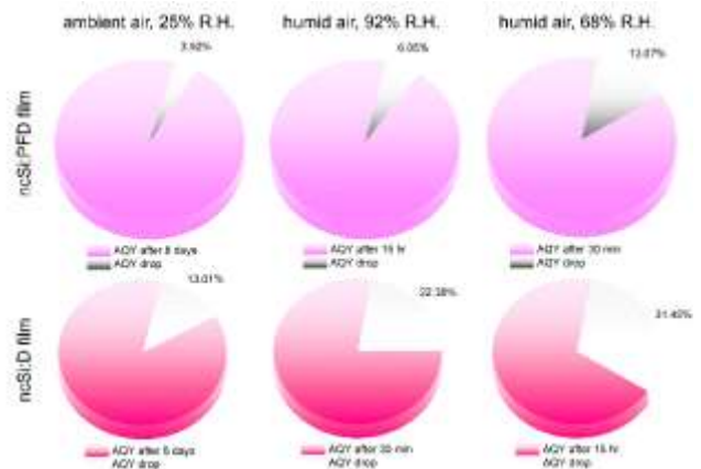
Figure 4. Comparison of the relative drop in absolute quantum yield (AQY) of two films under different conditions (area of the pies reflect the initial absolute values of AQY, 35% for ncSi:PFD film and 28% for ncSi:D film): top, ncSi:PFD film; bottom, ncSi:D film; left, exposed to air (R.H. 25%) for 8 days; middle, exposed to air (R.H. 92%) for 30 minutes; right, exposed to air (R.H. 68%) for 15 hours.
