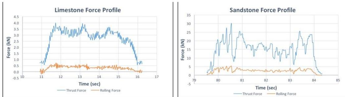
Figure 4: Typical force profile during cutting in limestone (left) and sandstone (right)
