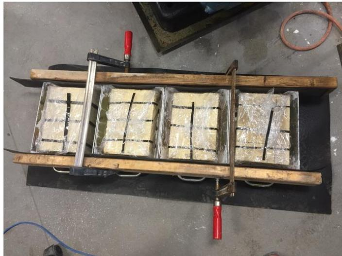
**Figure 1: Dry block samples wrapped in plastic and ready for casting**
