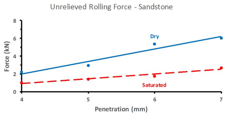
Figure 8: Variation in rolling force with depth in cutting sandstone.
