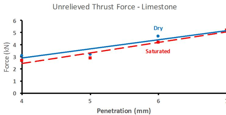
Figure 7: Variation in thrust force with depth in cutting limestone
