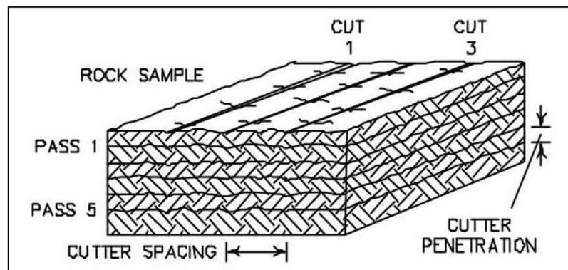
Figure 3: Schematic of the LRCM sample and nomenclature (Baldi, 2013).
