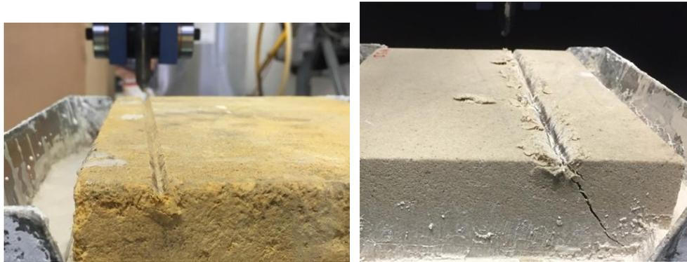
Figure 5: Localised crushing in limestone (left) compared to substantive rock chips in cutting sandstone (right)
