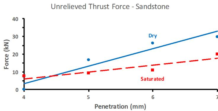
Figure 6: Variation in thrust force with depth in cutting sandstone
