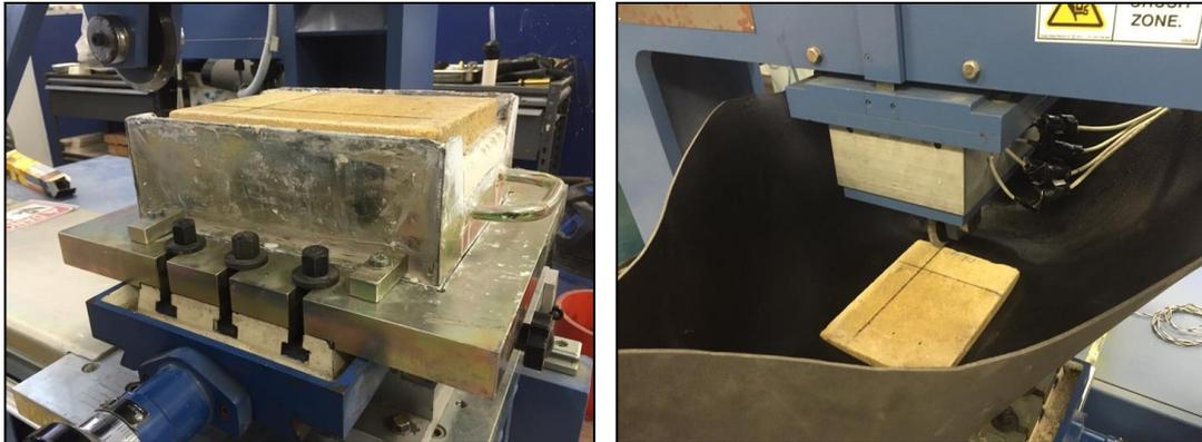
Figure 2: Block sample fastened to LRCM table prior to cutting (left) and foam containment structure to retain cutting debris (right)
