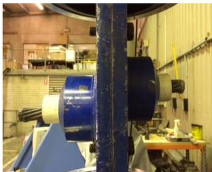
**Figure 4a: Single shear apparatus:**
