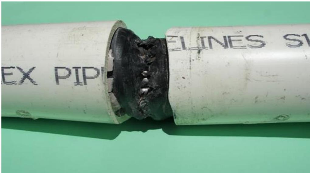
Figure 6: Damaged corrugated sleeve at the end of the shearing test
