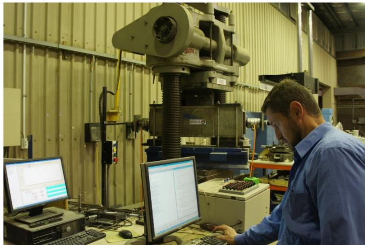
Figure 7: Double shear testing apparatus in 500 t compression testing machine
