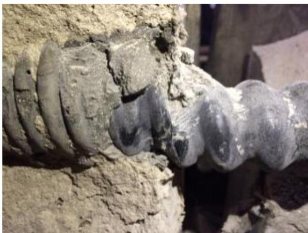
**Figure 9: Post-test pictures of double shearing for 20 mm of shear displacement**
