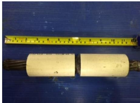
**Figure 4b: Cable section with corrugated sleeve installed in 45 mm plastic tube**
