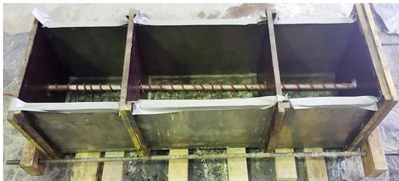
Figure 1: Concrete blocks casting assembly
