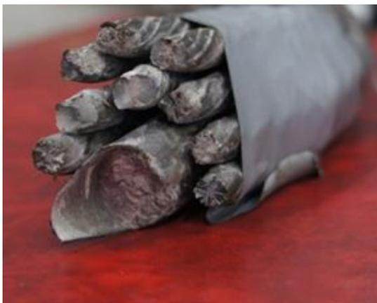
Figure 7: Tensile and shear failure of cable bolt
