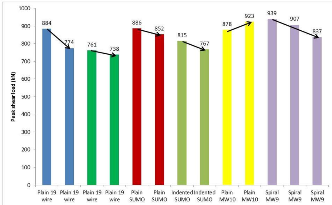
Figure 3: Effect of pretension load on peak shear load
