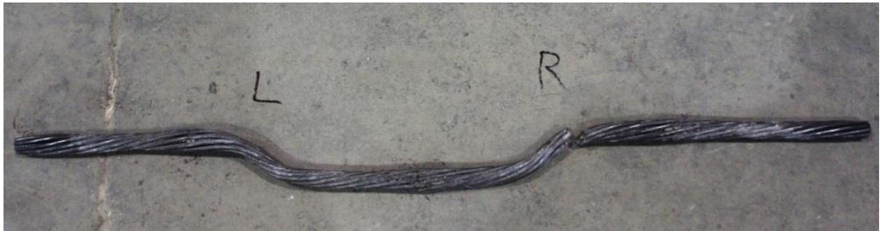
Figure 6: Failure angle of cable bolt
