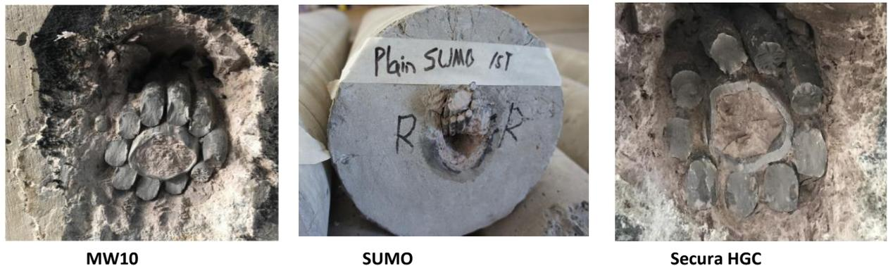
**Figure 5: Three shear tests for three different cables**
