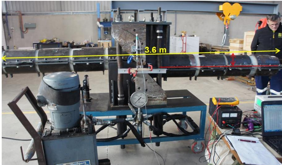
**Figure 1: Single shear test apparatus**
