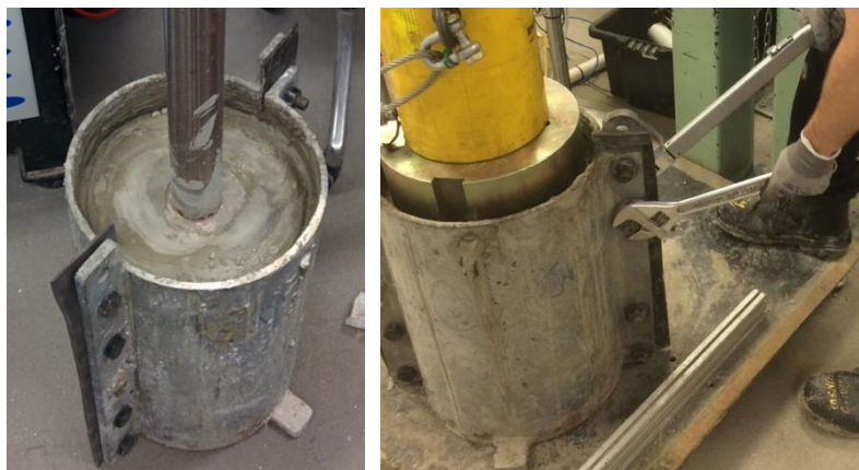
Figure 7: Confinement split-tubes grouted around sample (left); and, confinement torque being applied (right).
