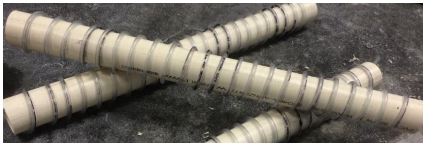
Figure 3: Silicone tubing wrapped around PVC pipe to create a consistent rifling effect in borehole
