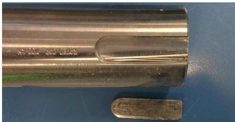
Figure 6: Machined anti-rotation key slot in the anchor tube (top) and, locking key (bottom)
