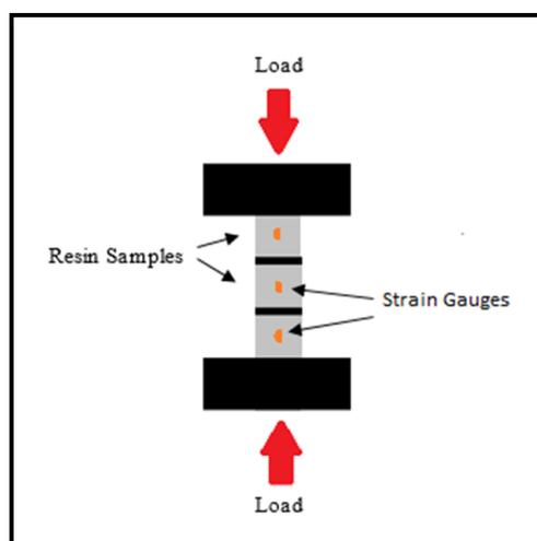
Figure 1: UCS test schematic
