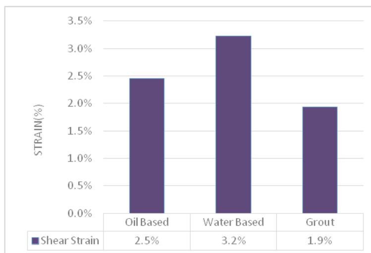
**Figure 10: Shear strain of bonding materials**
