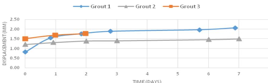
Figure 7: Pull test results for grout.
