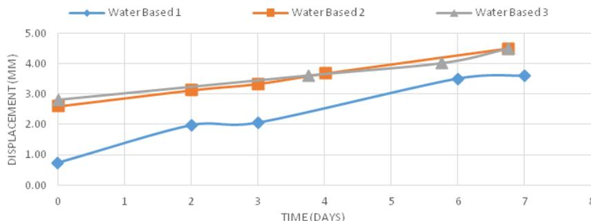
Figure 6: Pull test results for water based resin.
