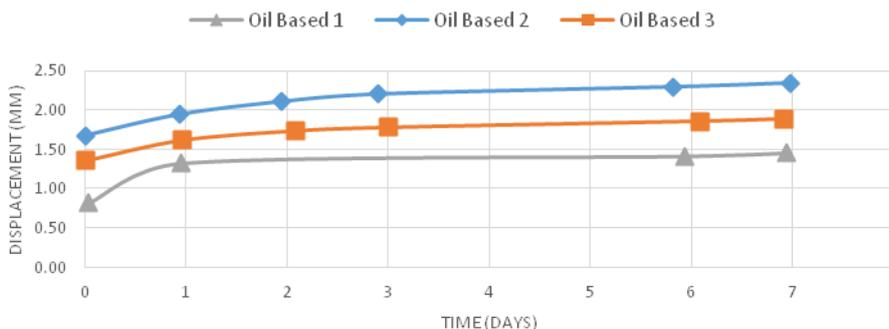
Figure 5: Pull test results for oil based resin
