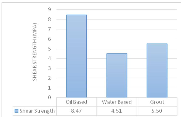
Figure 9: Shear strength of bonding materials
