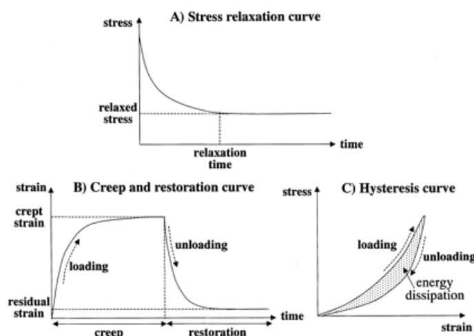
**Figure 4: Strain effects of loading and unloading on a material (Tanaka, 2003)**
