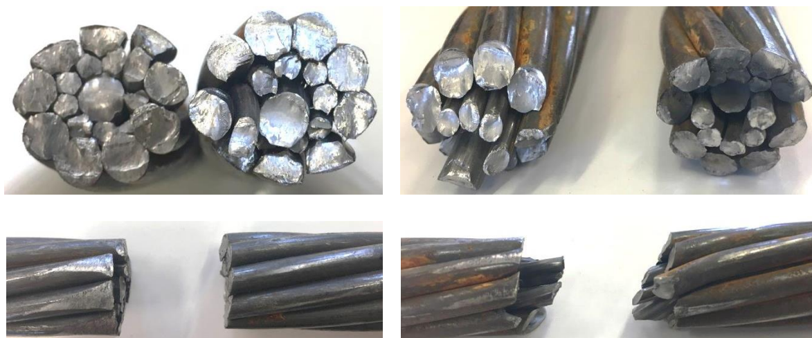
Figure 6: Typical high angle direct shear of 21.8 mm cable without pre-tension (left) and with 20 tonne pre-tension (right)
