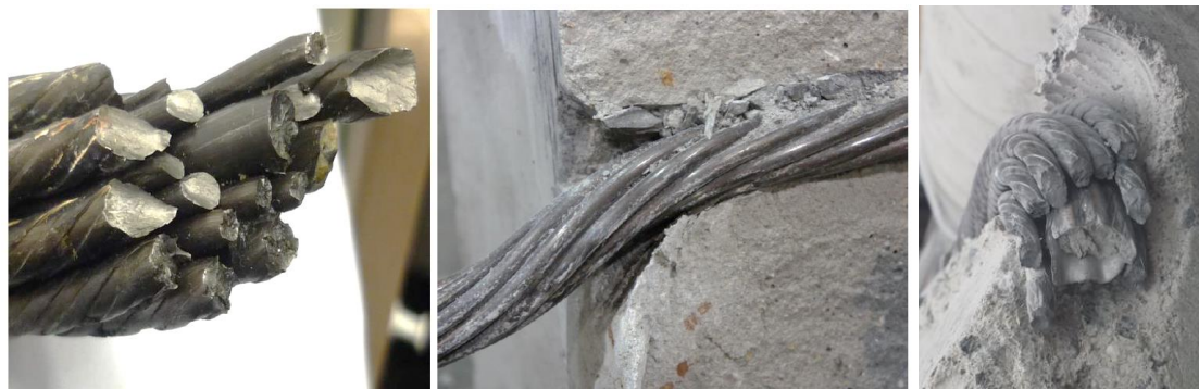
Figure 2: Cone and cup tensile failure of wires (left), and grout de-bonding and concrete block deformation during a double shear test (middle from Aziz et al , 2014), and bending and tensile failure during Megabolt Shear Testing (right from Megabolt, 2015)
