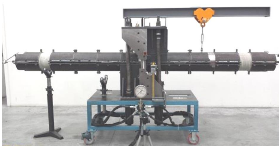
Figure 1: The Megabolt single shear test rig (Megabolt 2015)
