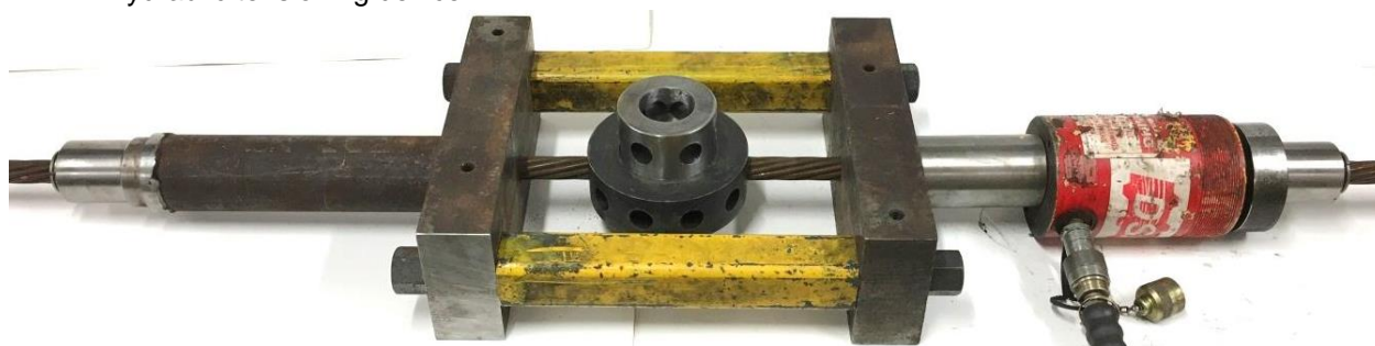
Figure 5: Cable pre tensioning frame – note the axially loaded cable does not increase loading on the shear plane surface
