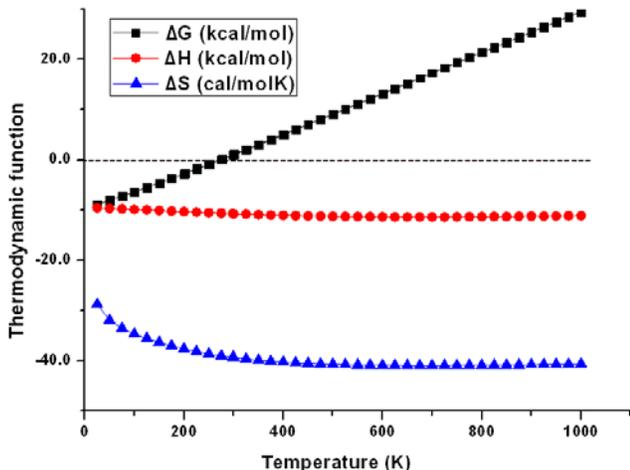
**Figure 4.** Variation of thermodynamic properties with temperatures (K) when an isolated  $N_2$  molecule is chemisorbed by  $1e^-$  charged  $B_{36}N_{36}$  in a type 1 configuration. Squares, triangles, and circles correspond to the change in Gibbs free energy (kcal/mol), change in entropy (cal/mol K), and change in enthalpy (kcal/mol), respectively.
