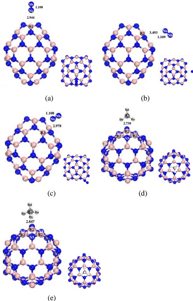
**Figure 1.** Top and side views of three physisorbed configurations: type 1 (a), type 2 (b), and type 3 (c) of N<sub>2</sub> on B<sub>36</sub>N<sub>36</sub> in its neutral state. Top and side views of two most stable configurations of CH<sub>4</sub> adsorption on B<sub>36</sub>N<sub>36</sub> in its neutral state (d, e). Atom color code: blue, nitrogen; pink, boron; gray, carbon; white, hydrogen.
