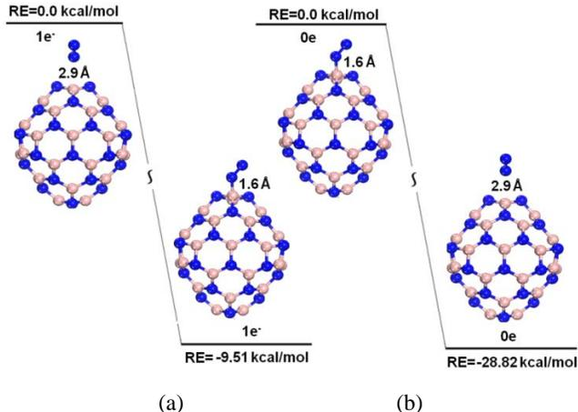
**Figure 5.** Energy change for reactions involving  $N_2$  adsorption on  $B_{36}N_{36}$  of type 1 (a) involves the change from physisorbed to chemisorbed configurations with the  $1e^-$  charged  $B_{36}N_{36}$ , respectively; (b) is the change from physisorbed to chemisorbed configurations with the neutral  $B_{36}N_{36}$ .
