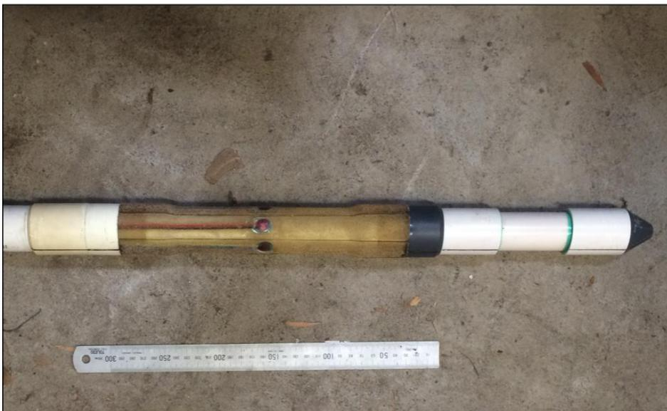
a) 48mm diameter ANZI strain cell.
