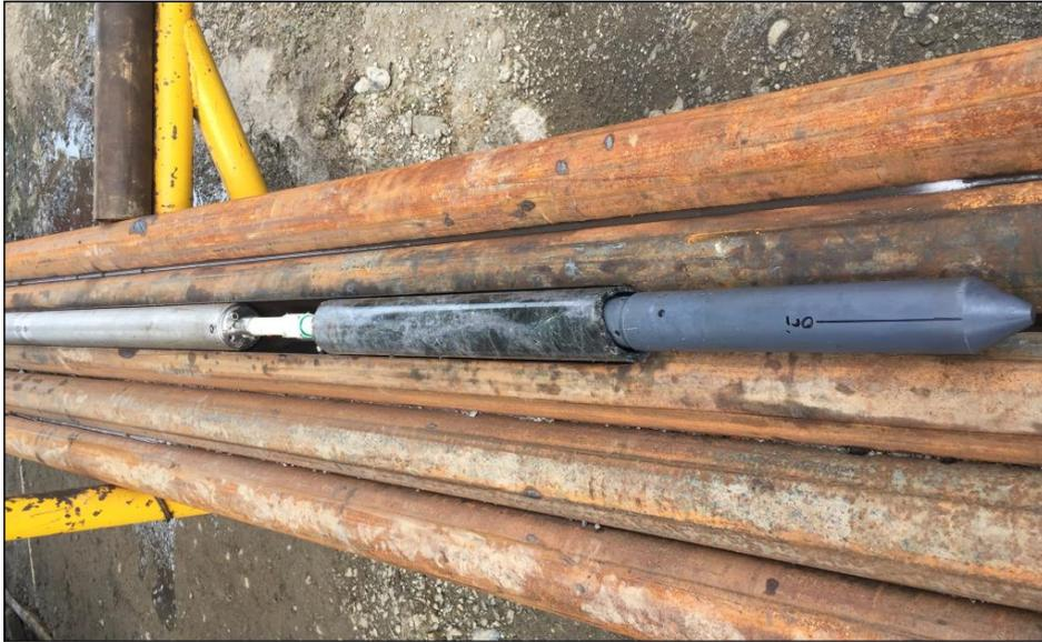
c) Downhole logger, recovered overcore and compass module.
