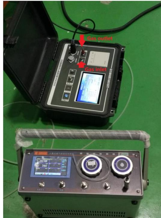
Fig. 7. The prototype of the proposed SF<sub>6</sub>/N<sub>2</sub> concentration detector.
