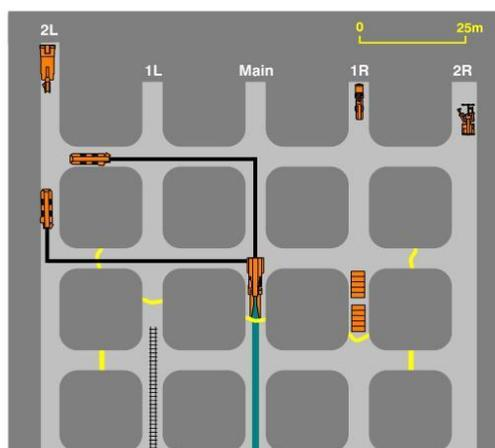
**Figure 3: Five heading mechanized continuous miner layout**
