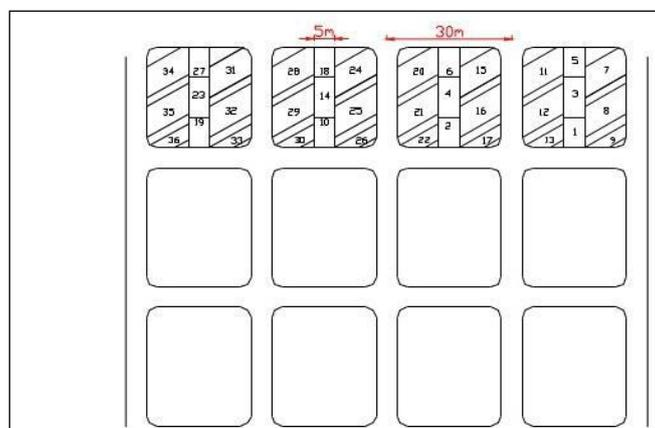
Figure 5: A typical cutting sequence for depillaring panel
