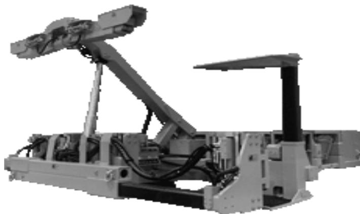
**Figure 2 A typical Joy Quad bolter (Multi-bolter)**
