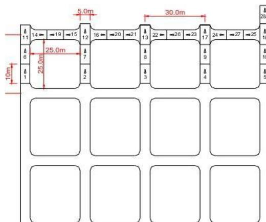
Figure 4: A typical cutting sequence for development panel
