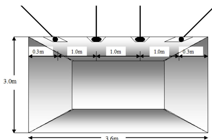
Figure 11: Support system design (3)
