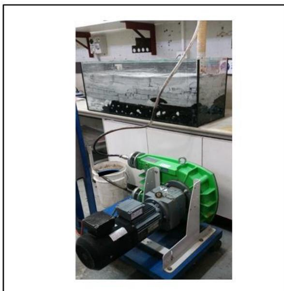
Figure 4: Connected laboratory scale injection system
