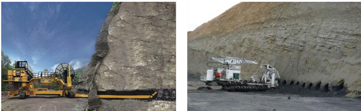
Figure 1: Highwall mining systems (a) CHM system (after Caterpillar Inc.), (b) Auger mining system (Coal Augering Services 2014)
