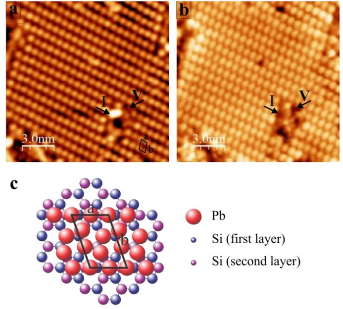
Fig.2. (a) STM height image, (b)  $dI/dV$ -image, and (c) structure model of the  $\sqrt{3} \times \sqrt{7}$  phase of a Pb thin film. Defects are indicated by “I” for impurity and “V” for vacancy. The unit cell corresponding to the atomic lattice is indicated in (a) and (c). ( $V = 1.4$  V,  $I = 0.1$  nA)
