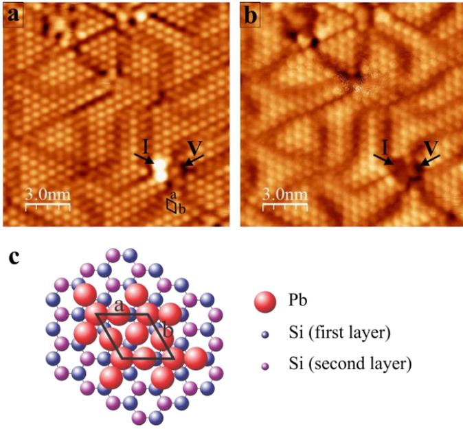
Fig.1. (a) STM height image, (b)  $dI/dV$ -image, and (c) structure model of the stripped incommensurate (SIC) phase of a Pb thin film. Defects are indicated by “I” for impurity and “V” for vacancy. The unit cell corresponding to the atomic lattice is indicated in (a) and (c). ( $V = 1.2$  V,  $I = 0.1$  nA)
