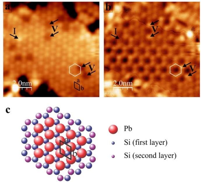
Fig.3. (a) STM height image, (b)  $dI/dV$ -image, and (c) structure model of the  $1 \times 1$  phase of a Pb thin film. Defects are indicated by “I” for impurity and “V” for vacancy. Two double vacancies are indicated. A white hexagon indicates the hexagonal atomic structure and LDOS. The unit cell corresponding to the atomic lattice is indicated in (a) and (c). ( $V = 1.6$  V,  $I = 0.1$  nA)
