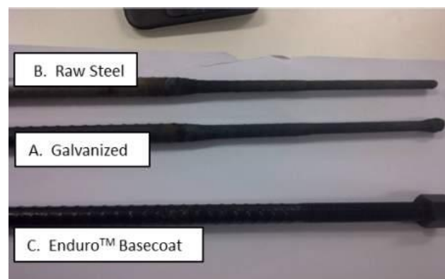
Figure 6: Acid bath immersion testing results after 50 days
