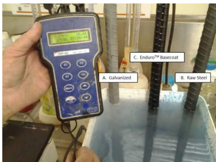
Figure 4: Acid bath and pH monitoring instrument used during Enduro™ product testing
