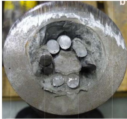
Figure 2: A view of the sheared sample, note the interaction between the strand and the steel tube
