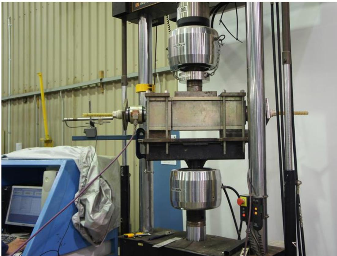
Figure 9: An assemble FG dowel with load cells for double shear testing in 50 t Instron testing machine
