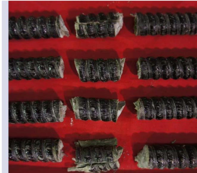
Figure 8: failure pattern of dowels in guillotine
