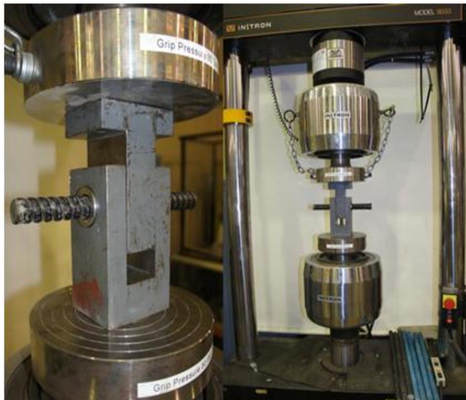
Figure 7: Double shear guillotine apparatus set up
