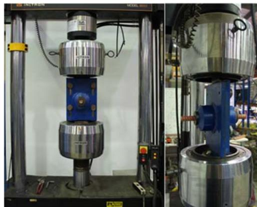
Figure 4: Single shear guillotine apparatus
