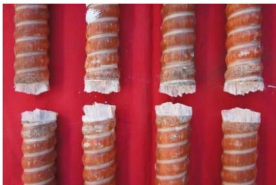
Figure 5: Single sheared failed 22 mm diameter dowels
