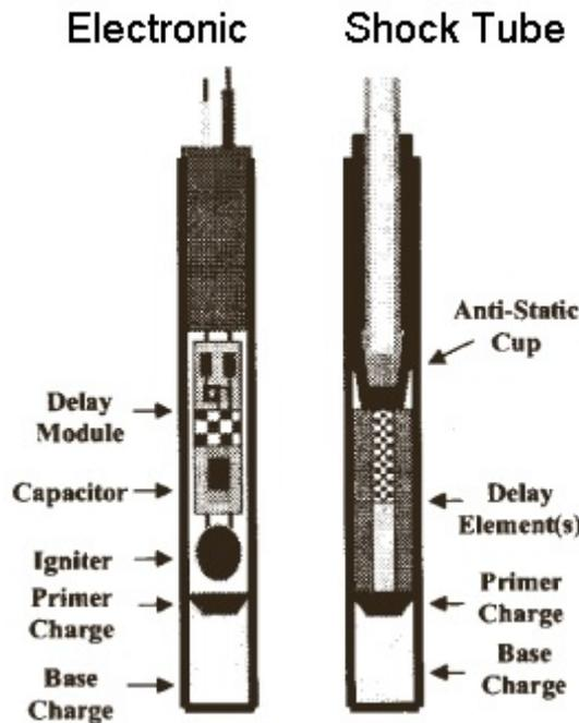
Figure 3: Detonators used on-site during the trial period (adapted from Coundouris and Scott, 2009)
