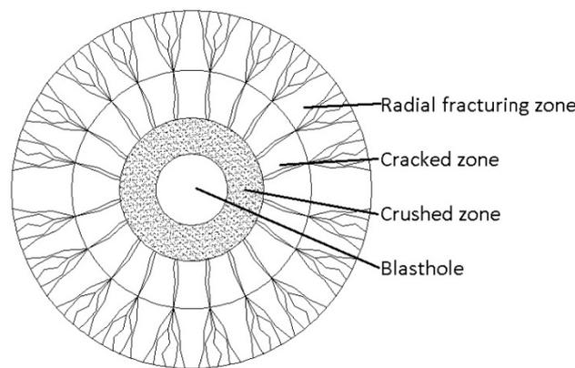
Figure 1: Zones of breakage around a blasthole
