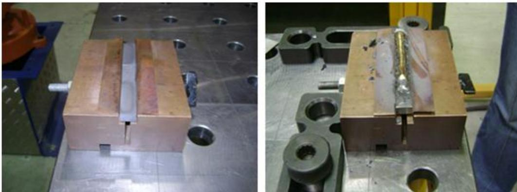
**Figure 3 Welding fixture with test piece assembly before the deposition of the single weld and immediately after deposition of test run.**
