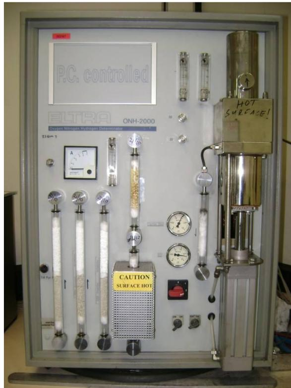
**Figure 5 Eltra ONH-2000 - Inert gas melt extraction test facility.**
