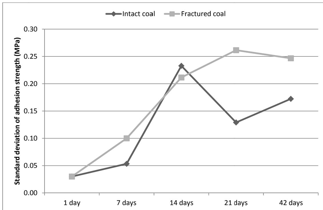
Figure 5: Standard deviation of adhesion strength with different curing time
