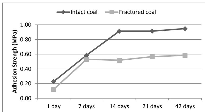
**Figure 4: Adhesion strength with different curing time**
