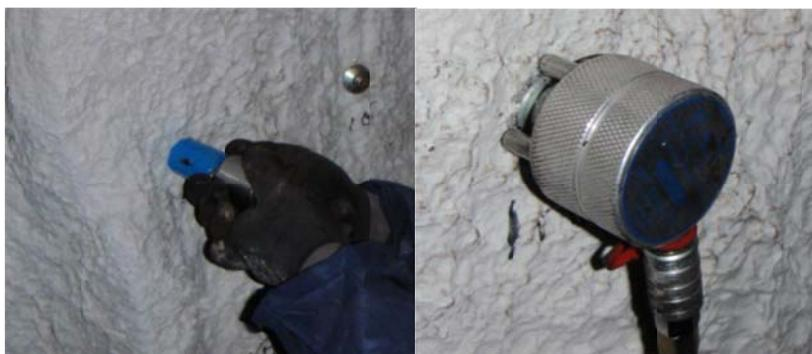
Figure 3: *In situ* adhesion strength test (a) overcoring, (b) dolly under test
