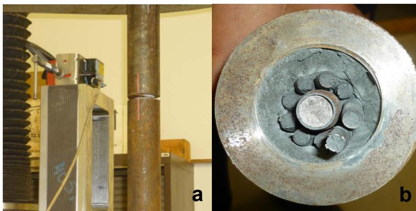
Figure4: (a) Tensile pull test set up and (b) snapped section of the cable bolt
