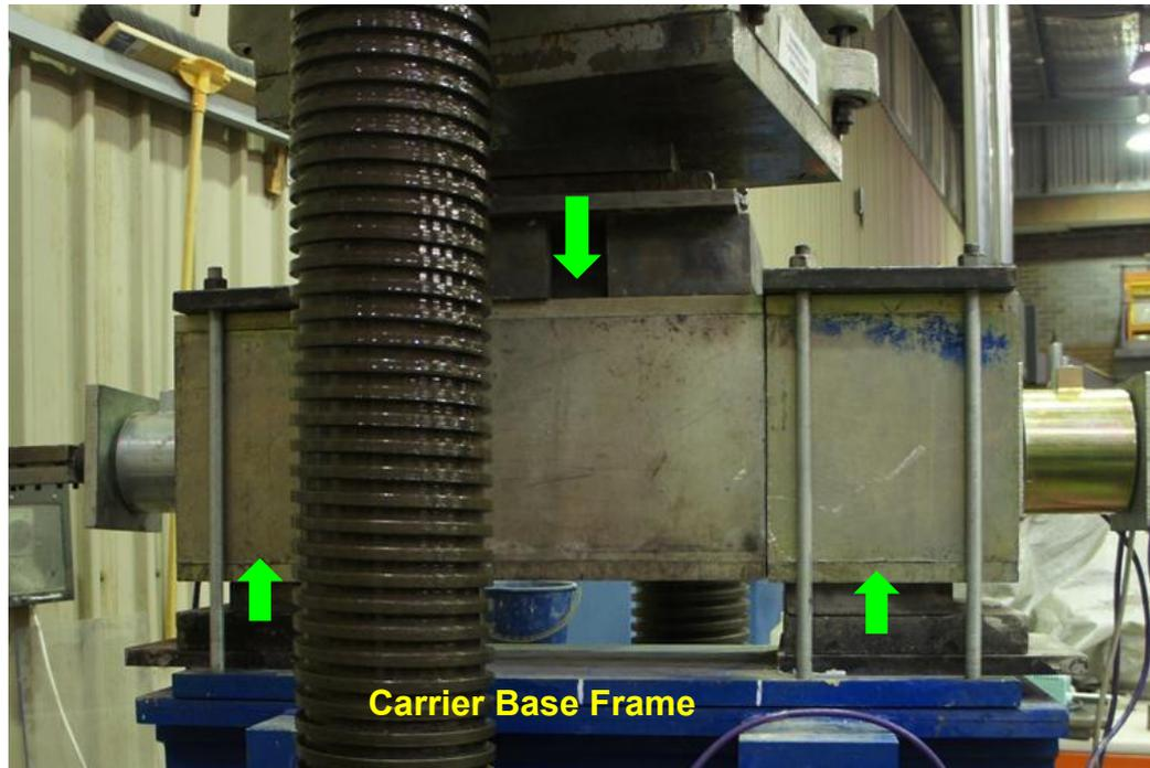
Figure 9: Double shear cable and concrete blocks assembly
