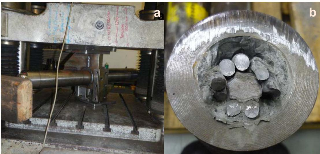
Figure 6: Shear test and a view of the sheared sample. Note the interaction between the strands and the steel tube
