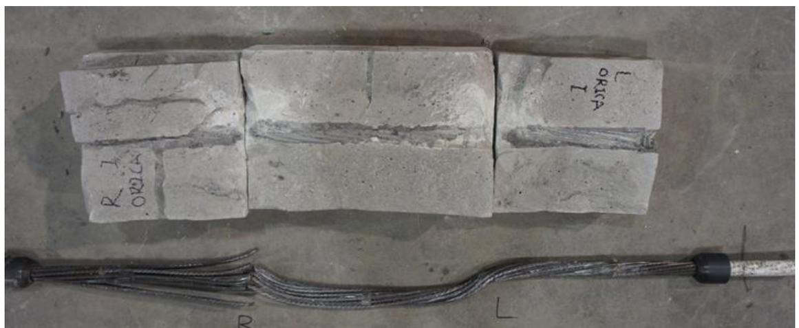
Figure 10: Post-test dismantled cable double shear assembly
