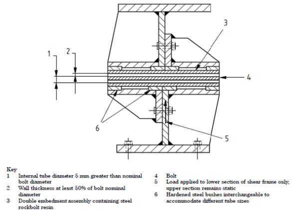
**Figure 1: Single shear frame for testing of cable bolt (BS7861- part 2: 2009)**
