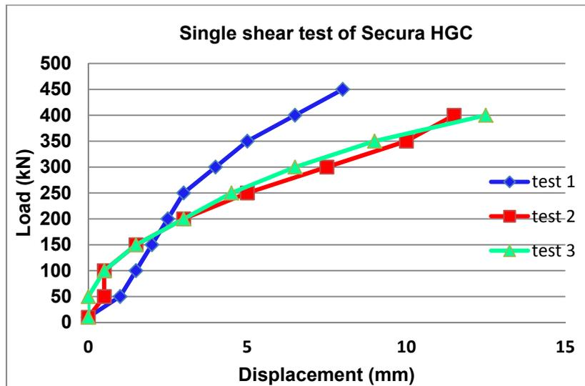
Figure 7: Load-displacement graphs of single shear tests
