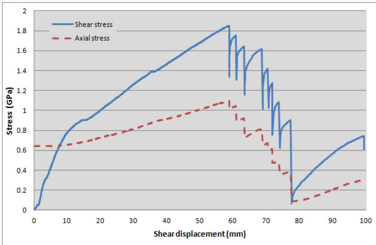
Figure 9: Shear behaviour of cabled concrete [test 4]
