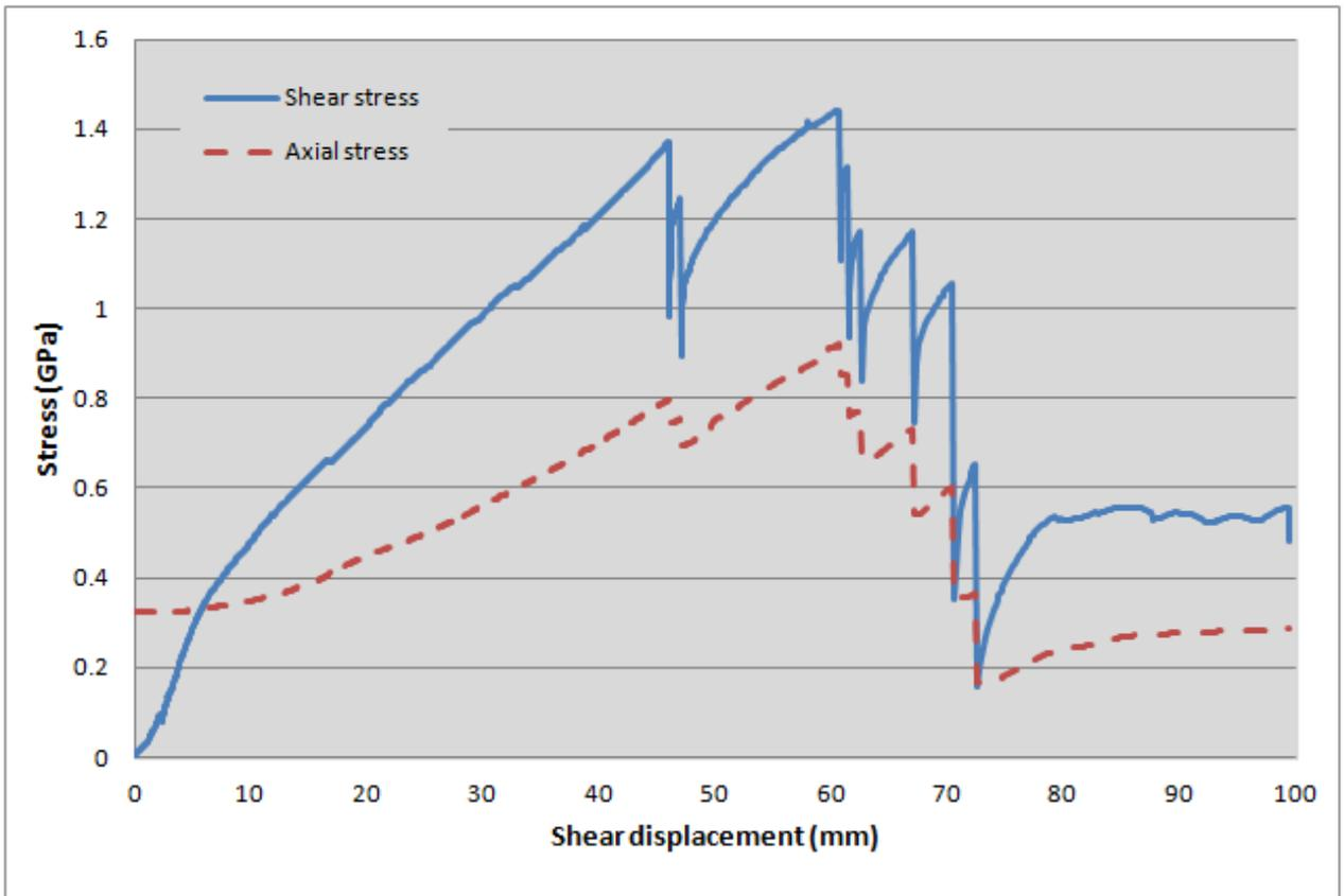
Figure 10: Shear behaviour of cabled concrete [test 5]
