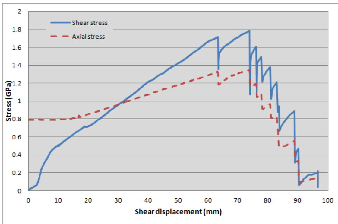
Figure 7: Shear behaviour of cabled concrete [test 2]
