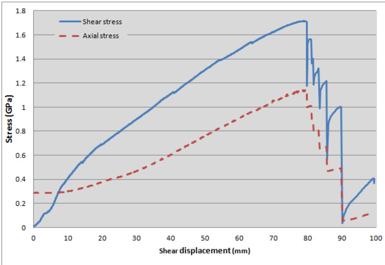
Figure 8: Shear behaviour of cabled concrete [test 3]
