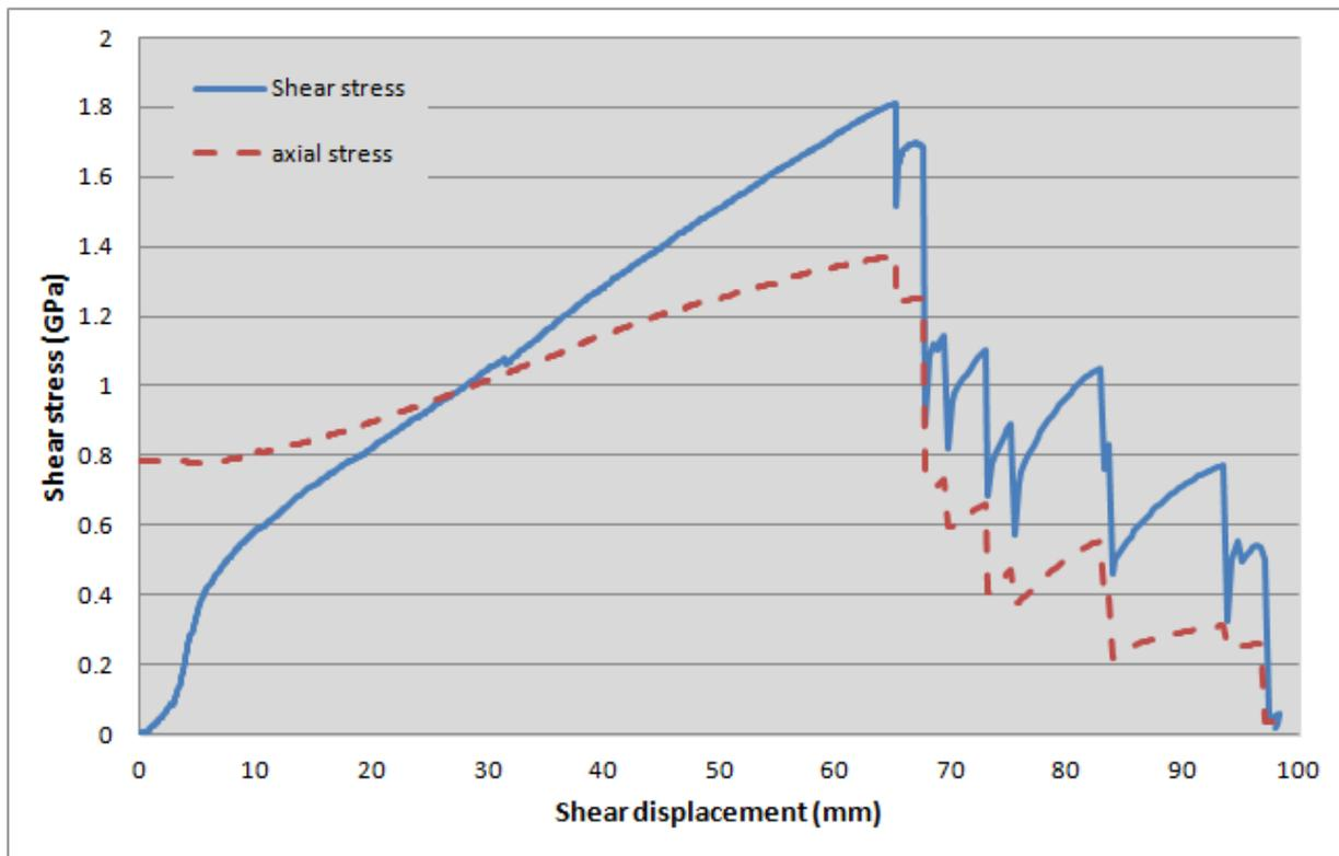
Figure 12: Shear behaviour of cabled concrete [test 7]
