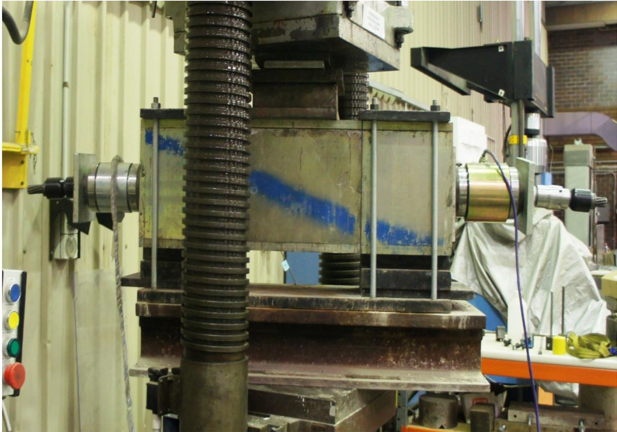
**Figure 4: Arrangement of shearing apparatus on compression machine**
