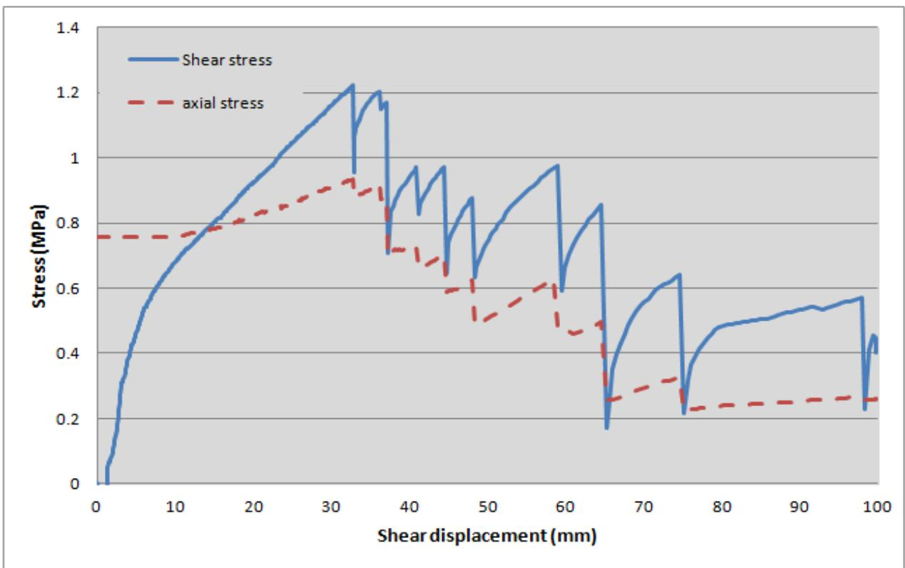
Figure 11: Shear behaviour of cabled concrete [test 6]
