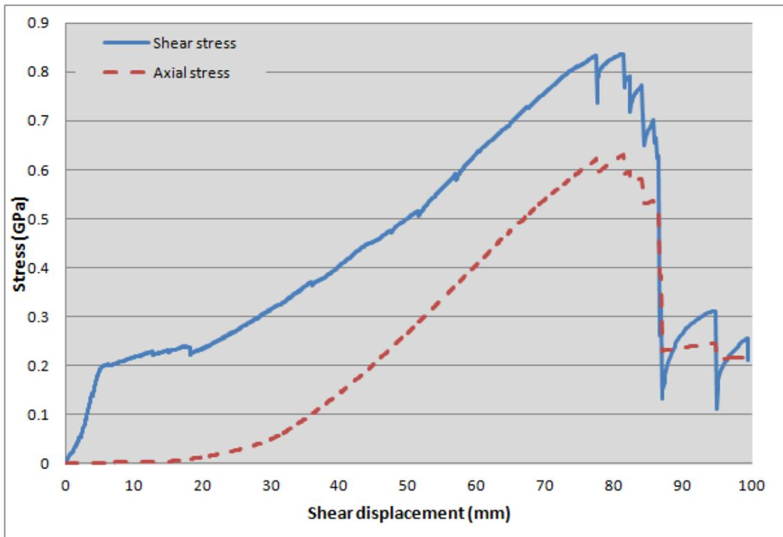
Figure 6: Shear behaviour of cabled concrete [test 1]
