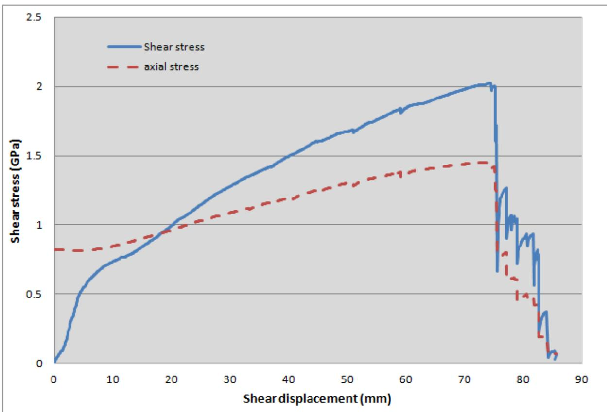
Figure 13: Shear behaviour of cabled concrete [test 8]
