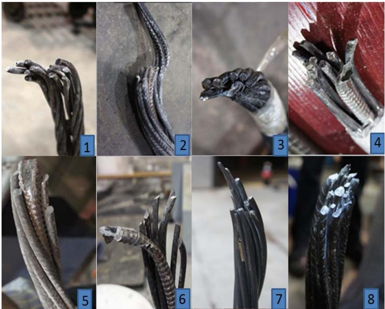
Figure 14: strands snapped of the tested cables
