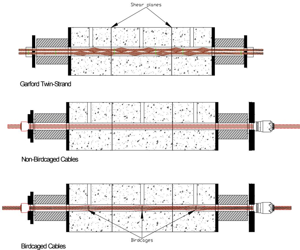
Figure 3: Cross section of double shear blocks and cables
