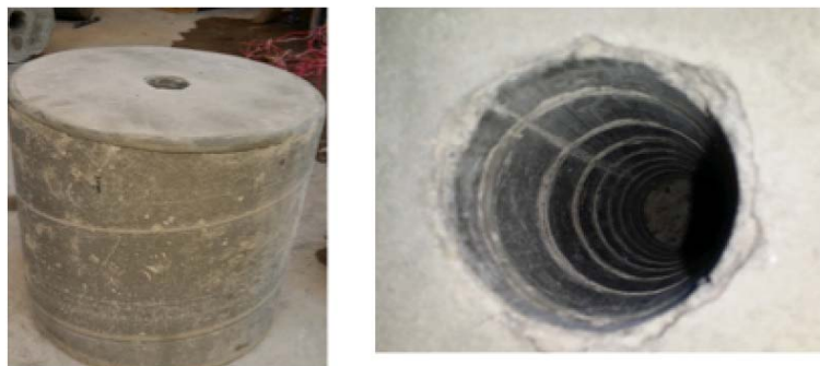
Figure 6: Test sample (left) with rifling borehole (right)
