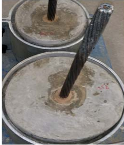
Figure 8: Cable bolt embedded in test sample using a slow set resin
