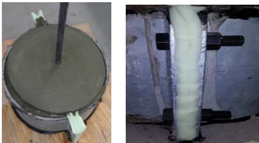
Figure 10: a) Test sample placed in assembled steel cylinder (left) and b) gap filled with foam and bolts on side of cylinder that were tensioned before a test (right)
