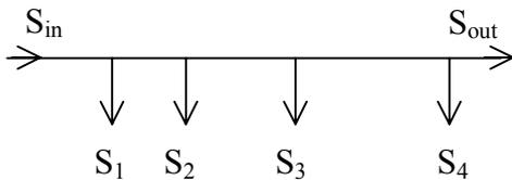
Figure 2 - MV feeder with several take-off points.
