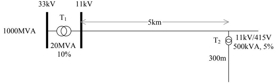
Figure 4 - Example showing MV and LV levels
