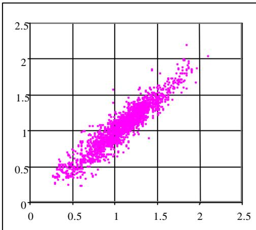
Fig.10: Scattergraph of 5<sup>th</sup> harmonic voltages  $V_a$  versus  $V_c$  at Site 5 (Residential LV)
