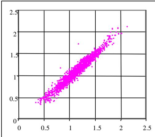
Fig.9: Scattergraph of 5<sup>th</sup> harmonic voltages  $V_{ab}$  versus  $V_{cb}$  at Homepride zone substation
