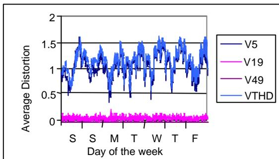
Fig. 4: Homepride Zone Substation 11kV harmonic voltage trend
