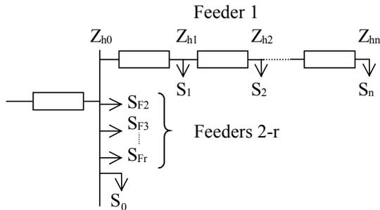
Figure 1: Example radial MV distribution system
