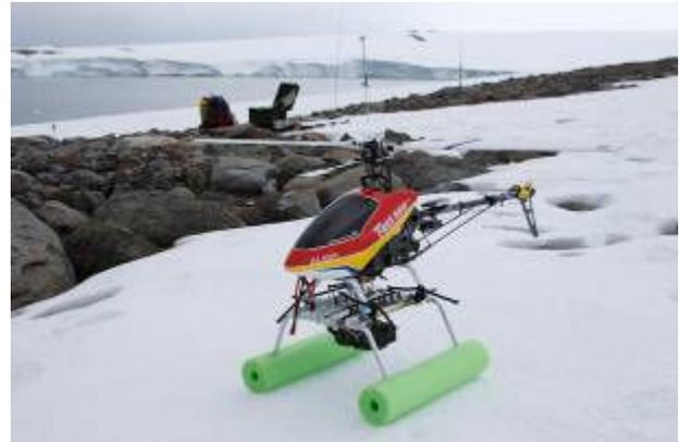
Figure 3. Our micro-UAV at the study site mounted with a camera, GPS receiver, and flight stabiliser.
