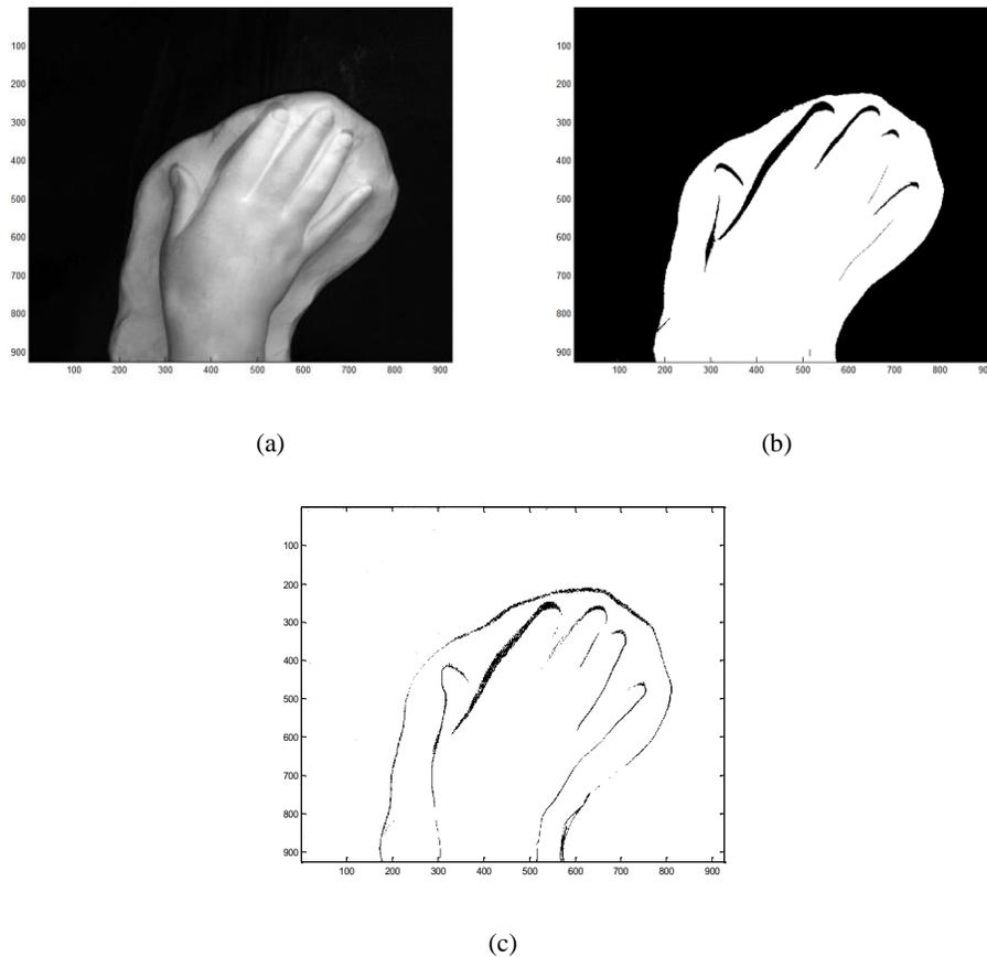
Figure 3(a) The object image. (b) The corresponding validation mask  $B(x, y)$  when  $I_{th} = 50$ , black indicates shadow pixels, white indicates pixels corresponding to object surface. (c) The identification of LQ pixels (black).
