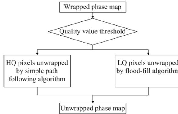
Figure 1 The flow-chart of our proposed method.
