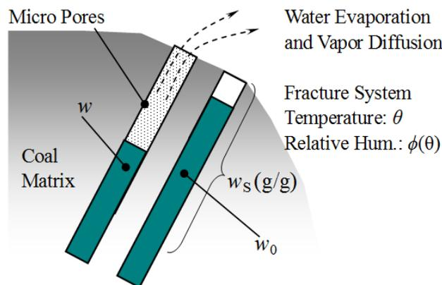
**Figure 6 - Model of moisture saturation in micro-pores of low-rank coal matrix**
