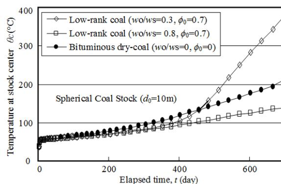
Figure 8 - Temperature-time curves at the centre in pile of bituminous and low-rank coals
