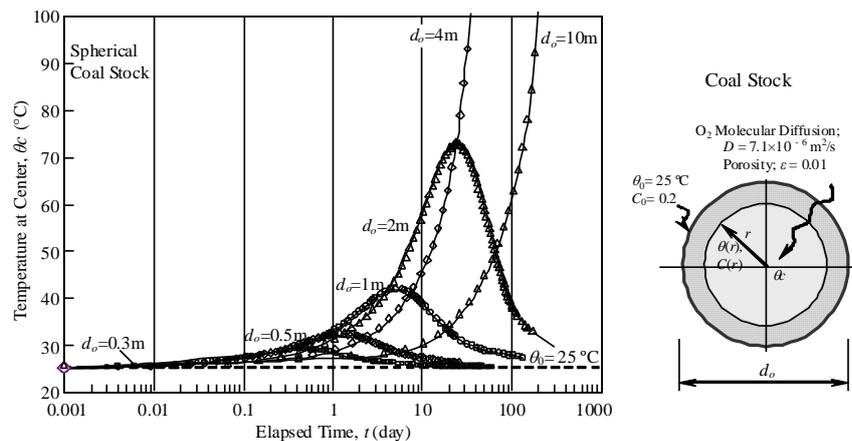
Figure 7 - Numerical simulation results on centre temperature of spherical coal stockpile of bituminous dry-coal with different diameter,  $d_0$  (m) (Tables 1 and 2)
