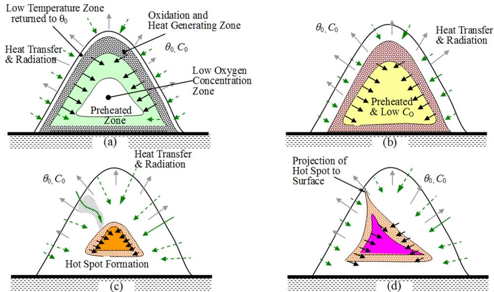
Figure 1 - Schematic figure showing self-ignition process of coal stockpile (Sasaki and Sugai, 2011)
