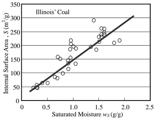
**Figure 4 - Model of the relationship between saturated moisture and internal surface area of low rank coal (see Thomas and Damberger, 1976)**
