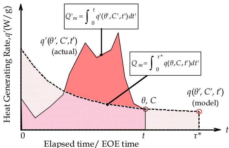
Figure 3 - Schematic definition of EOE-time of bituminous dry-coal to estimate heat generating rate by matching total heat generations (Sasaki and Sugai, 2011)
