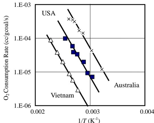
Figure 2 -  $\text{O}_2$  consumption rate of coals vs. inverse of absolute temperature measured by Kaji et al. (1987) (Coal samples were mined in USA, Australia and Vietnam)
