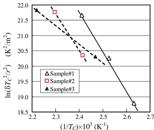
Figure 4 - Plotting  $\ln(\delta T_c^2/r^2)$  against  $(T_c)^{-1}$  based on critical self-ignition temperature (CSIT), showing results for different mesh-box sizes
