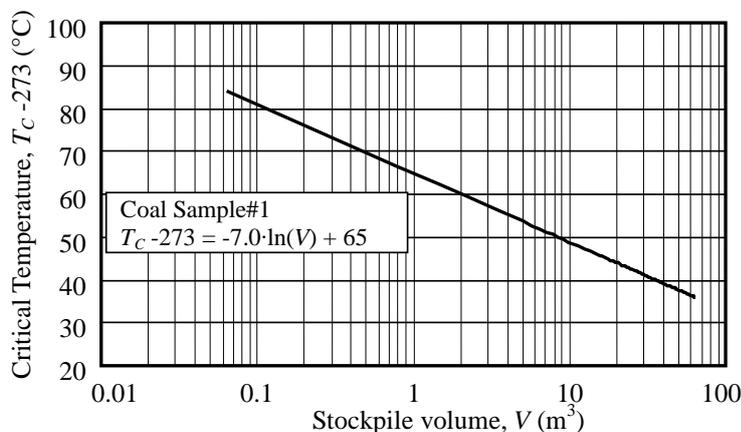
Figure 5 - A typical estimation of critical self-ignition temperature (CSIT) vs. corresponding to stockpile volume (Sample #1)
