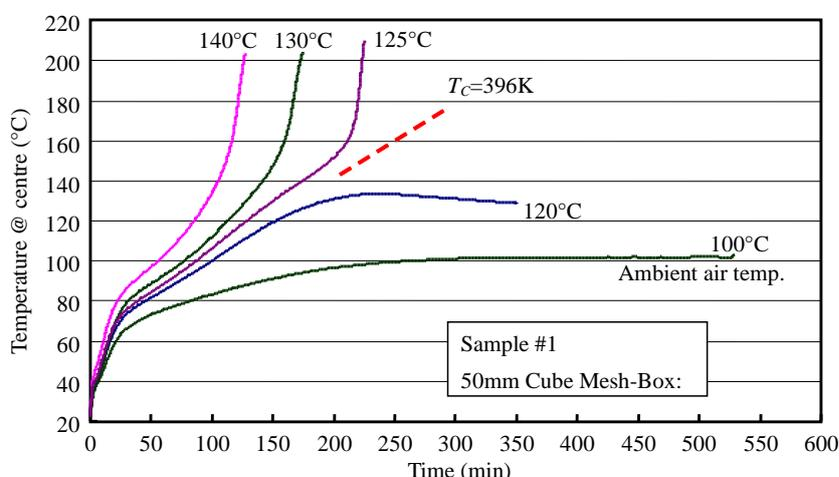
Figure 3 - Examples of temperature profiles for sample #1 at different ambient air temperatures at centre of 50mm cube mesh-box)
