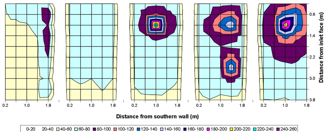
**Figure 1 - Hot spot development in 16 tonne reactor (Cliff, *et al.*, 2000a)**
