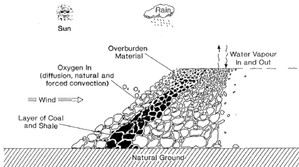
Figure 4 - Schematic representation of a spoil pile (from Carras, *et al.*, 1994) as reported in Day (2008)
