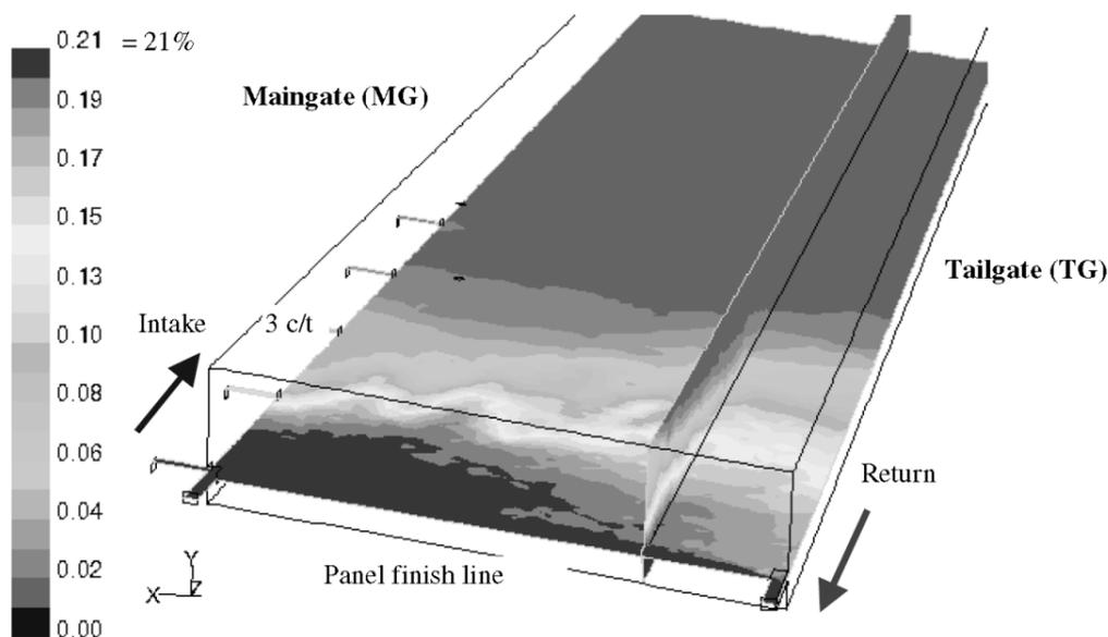
**Figure 2 - Oxygen gas distribution in the longwall goaf near the finish line – with 50 m<sup>3</sup>/s airflow (Balusu, *et al.*, 2002)**
