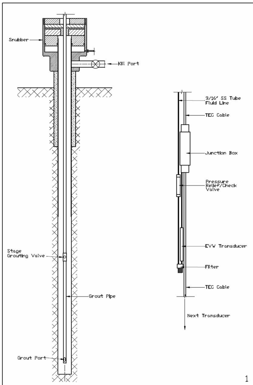
**Figure 2 - Stage grouted cemented transducer installation with details of transducer system for cement displacement on right**
