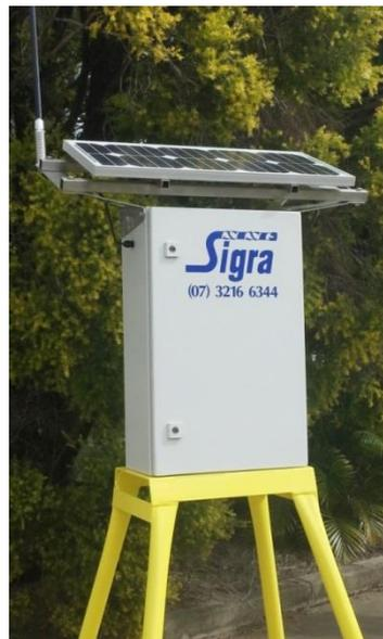
Figure 4 - Data acquisition system with logger box and modem
