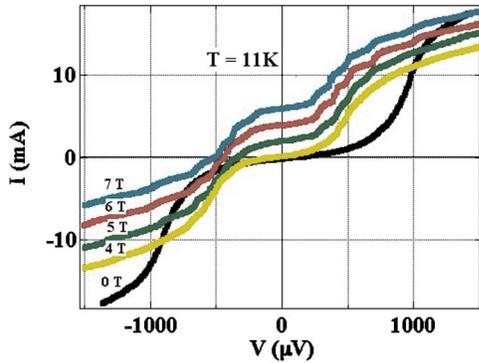
FIG. 1. (Color online)  $I$ - $V$  characteristics at 11 K and applied magnetic fields of 0, 4, 5, 6, and 7 T in the  $ab$  plane for a  $c$ -axis NBCO/PBCO/NBCO tunneling junction (Sample SNP1). The curves at 5, 6, and 7 T have been displaced vertically for clarity.
