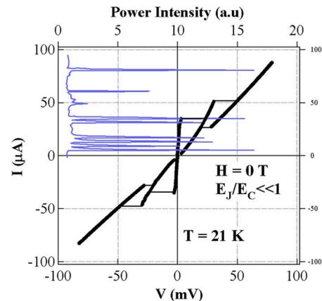
FIG. 3. (Color online)  $I$ - $V$  characteristics at 21 K for a NBCO/PBCO/NBCO tunneling junction (Sample SNP2) with the corresponding detected Josephson microwave power shown for a receiving frequency of 36 GHz. Here  $E_J/E_C \ll 1$ .
