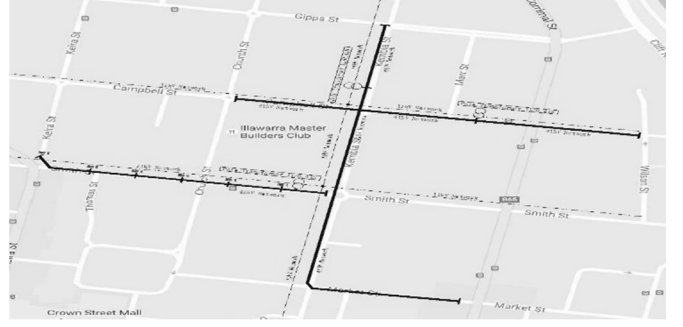
Fig. 2. Map of a part of 11kV and LV residential distribution networks in Wollongong City [22]
