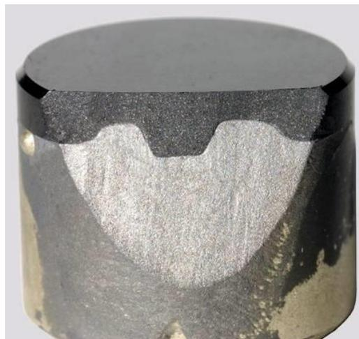
Figure 10 - Progressive wear of a PCD cutter
