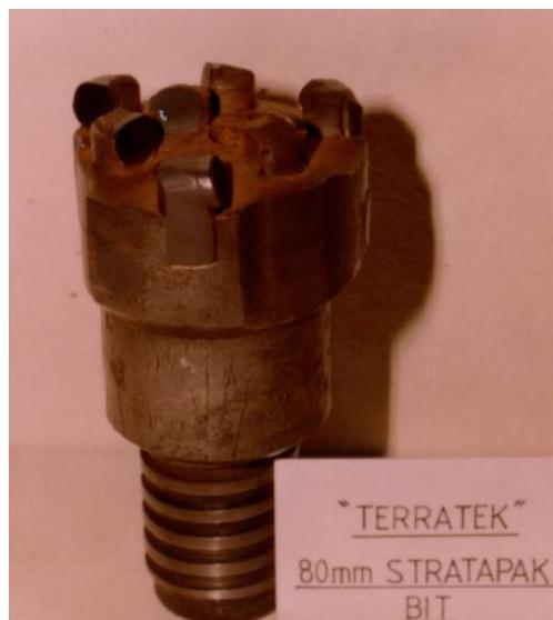
Figure 1 - “Terratek” 80 mm Stratapax PCD bit (Allen, 1982)
