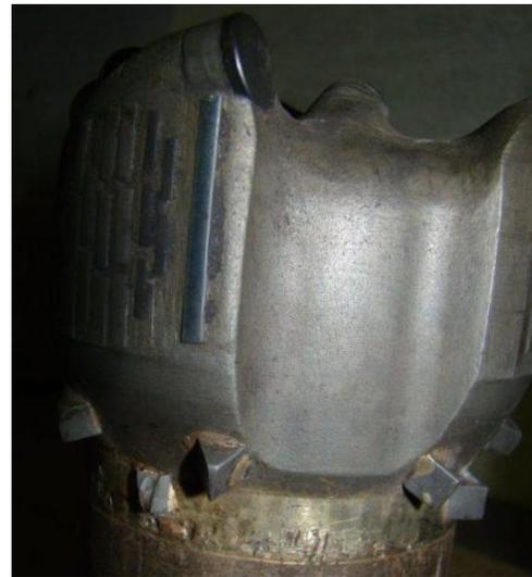
Figure 21 - Asahi PCD bit with tungsten carbide back-cutters
