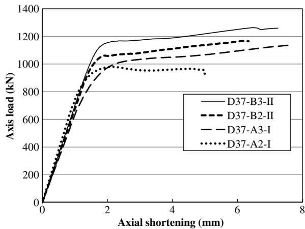
Fig. 5. Typical axial load-strain curves of DSTCs
