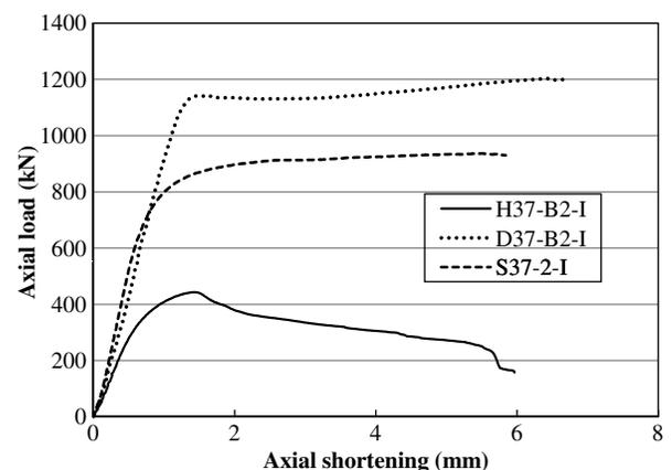
**Fig. 4.** Typical axial load-shortening curves
