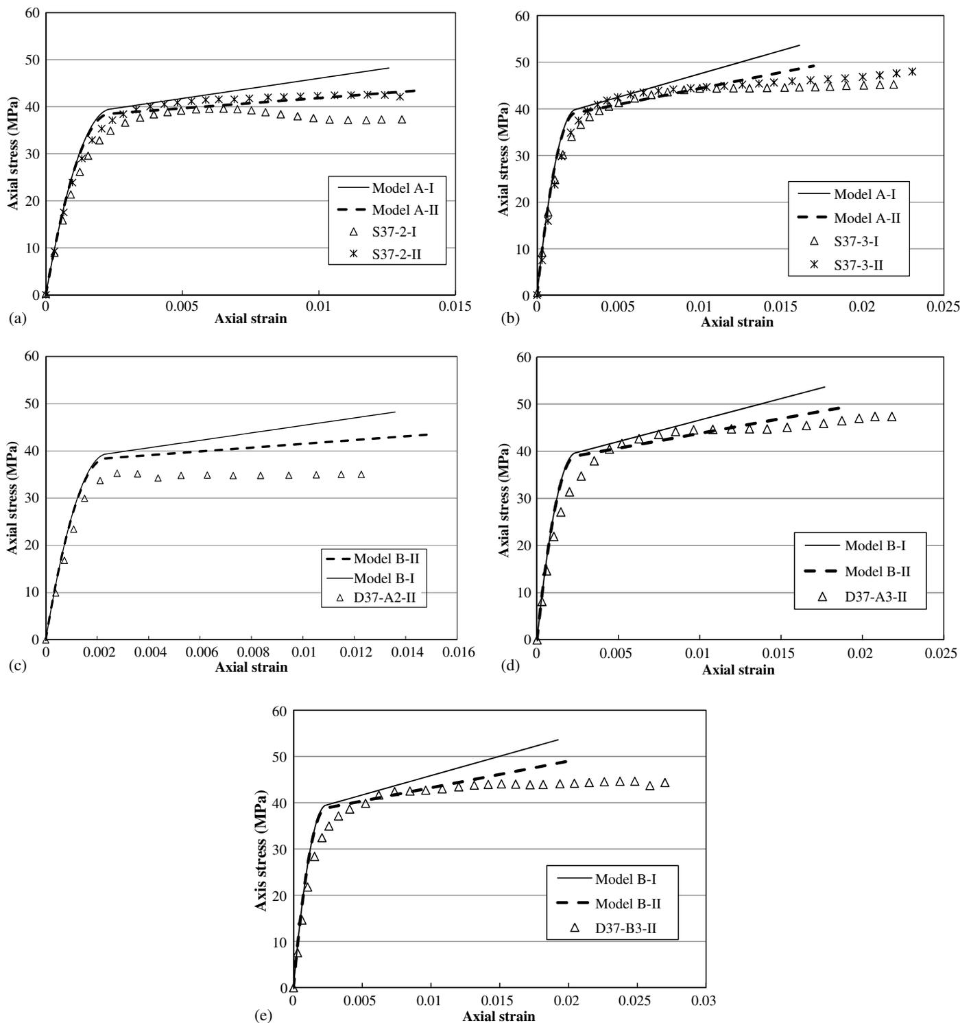
**Fig. 9.** Axial stress-strain curves: (a) FCSC specimens with a two-ply FRP jacket; (b) FCSC specimens with a three-ply FRP jacket; (c) specimen D37-A2-II; (d) specimen D37-A3-II; (e) specimen D37-B3-II
