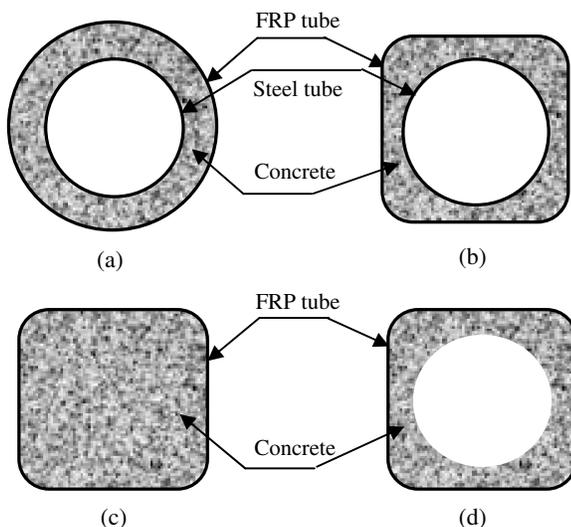
**Fig. 1.** Cross sections of hybrid DSTCs, FCSCs, and FCHCs: (a) circular hybrid DSTCs; (b) square hybrid DSTCs with a square FRP outer tube and a circular steel inner tube; (c) square FCSCs; (d) square FCHCs with a circular inner void
