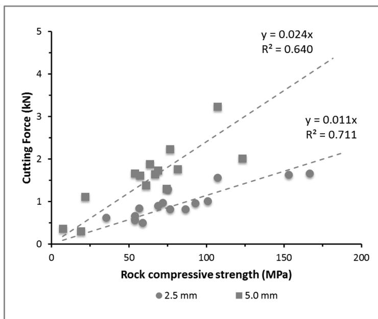
Figure 5 - Variation in cutting force with rock strength at two levels of cutting depth
