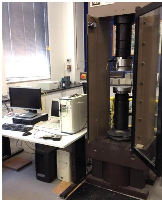
**Figure 3 - The MTS machine setup for the compressive strength tests**
