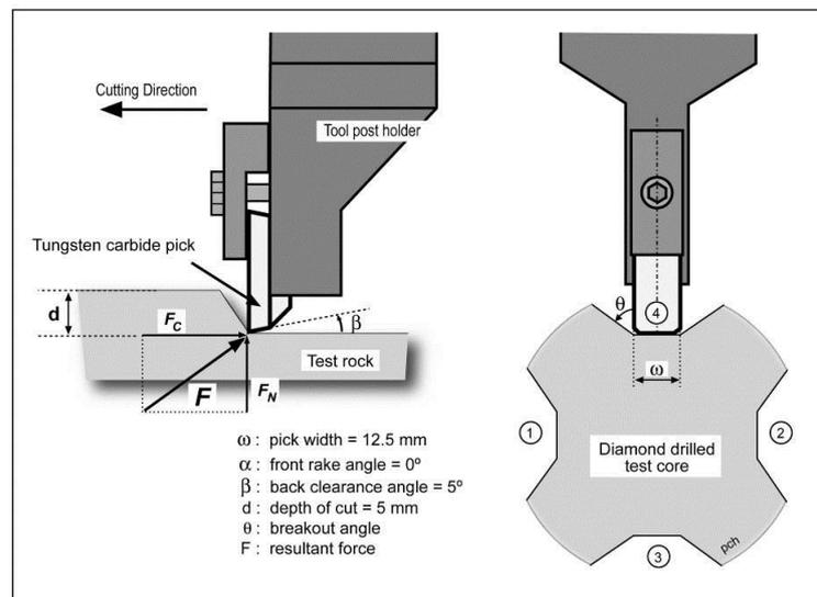
**Figure 1 - Schematic of the main variables in the core cuttability test procedure (Hagan, 1990)**
