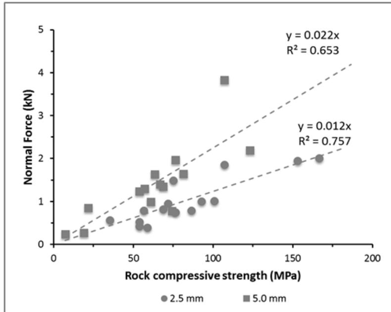
**Figure 6 - Variation in normal force with rock strength at two levels of cutting depth**
