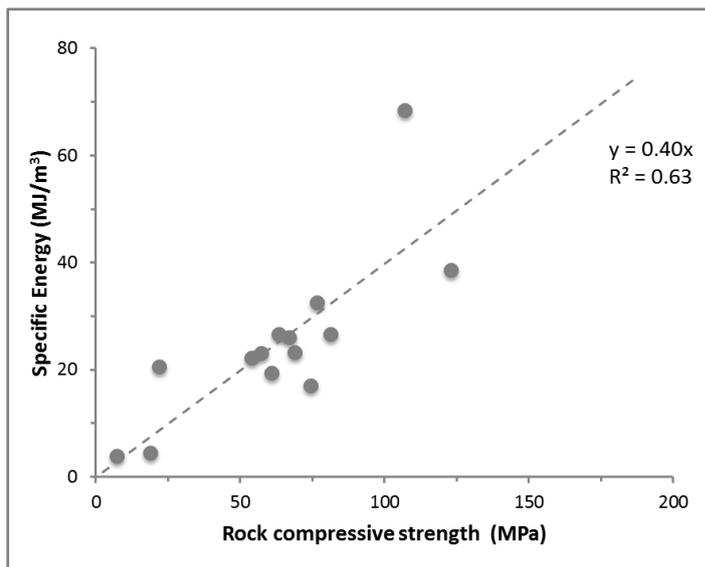
Figure 4 - Variation in specific energy with rock strength
