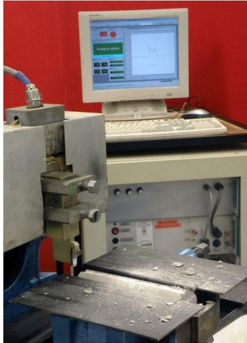
**Figure 2 - Cutting tool, dynamometer and data acquisition system used in the core cuttability test procedure at UNSW**
