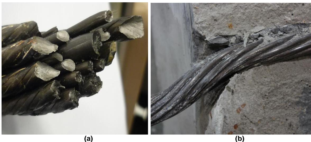
**Figure 6 - (a) failed indented strand cable bolt and (b) concrete deformation around sheared section of the bolt**
