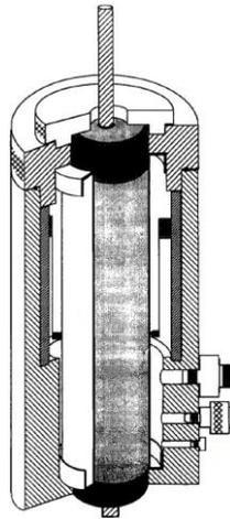
**Figure 3 - Cutaway section of a modified Hoek cell (after Macsporrán, 1993)**
