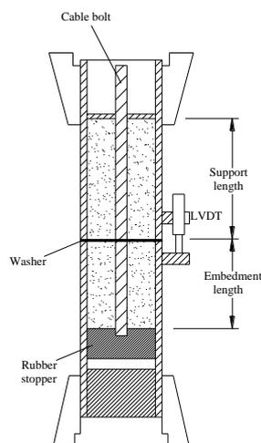
Figure 1 - Split-pulling rig (after Fuller and Cox, 1975)
