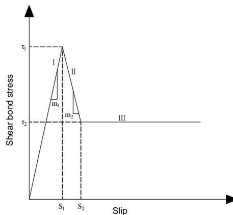
Figure 5 - Tri-linear bond stress-slippage model (after Benmokrane, et al., 1995)
