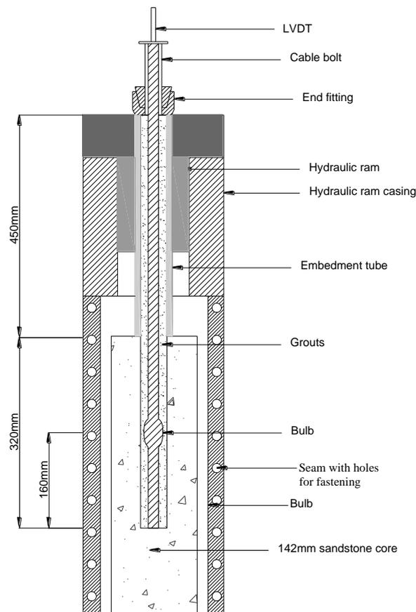
Figure 8 - Schematic diagram of modified LSEPT (after Thomas, 2012)
