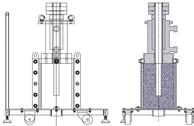
Figure 9 - Schematic of the design of proposed new LSEPT test facility
