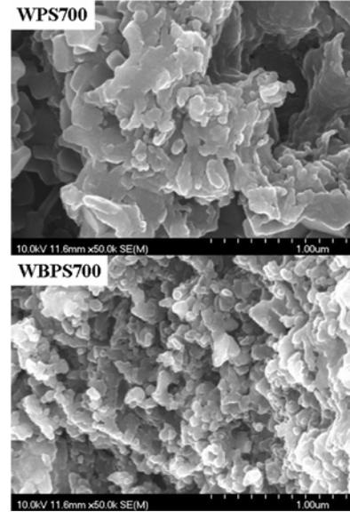
Fig. 4. Scanning electron microscope (SEM) images for (top) wire sample prepared from as-supplied boron, and (bottom) wire sample prepared from ball-milled boron. All samples were sintered at 700°C for 30 minutes.
