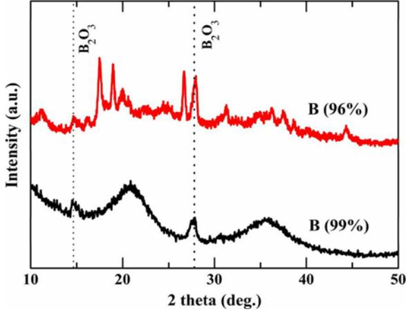
Fig. 1. XRD patterns for different boron powders.
