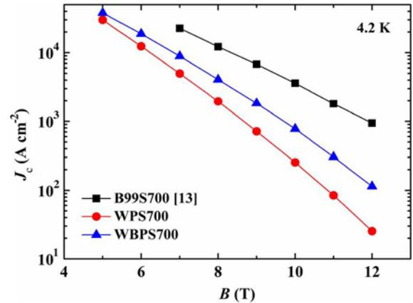
Fig. 5. Transport critical current density ( $J_{ct}$ ) for  $MgB_2$  wires as a function of external magnetic field at 4.2 K B99S700 is the reference sample from 99% B.
