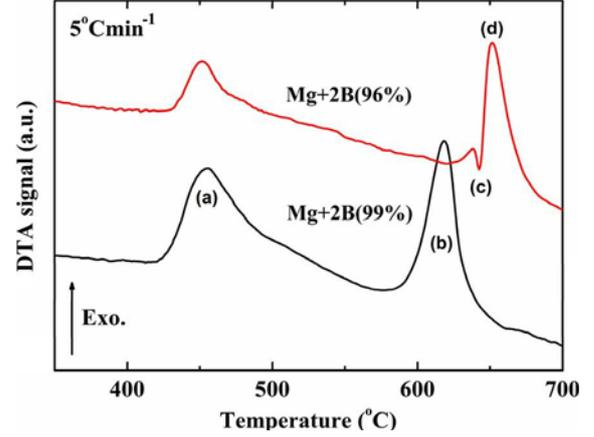
Fig. 2. Differential thermal analysis for  $\text{MgB}_2$  with different boron powders.
