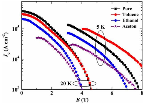
Fig. 3. The magnetic critical current density ( $J_{cm}$ ) as a function of field for the  $MgB_2$  samples [10].
